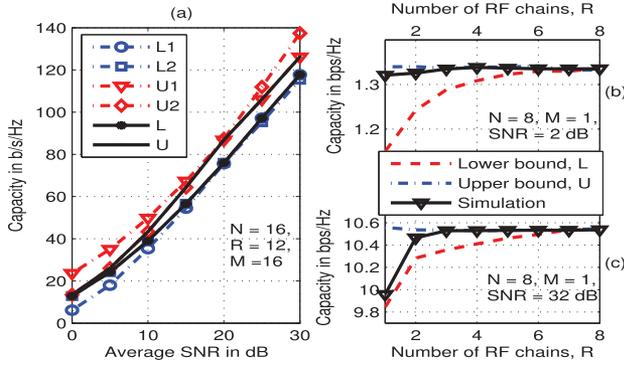
Fig. 1. Capacity bounds for different GSM-MIMO configurations.
