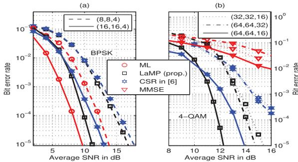
Fig. 3. BER performance comparison between proposed LaMP detection, CSR detection in [6], MMSE detection, and ML detection.
