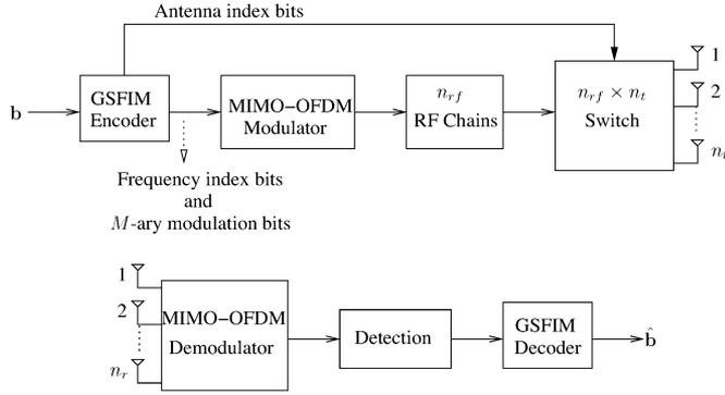
Fig. 8. Block diagram of GSFIM transmitter and receiver.
