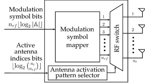
Fig. 1. GSIM transmitter.
