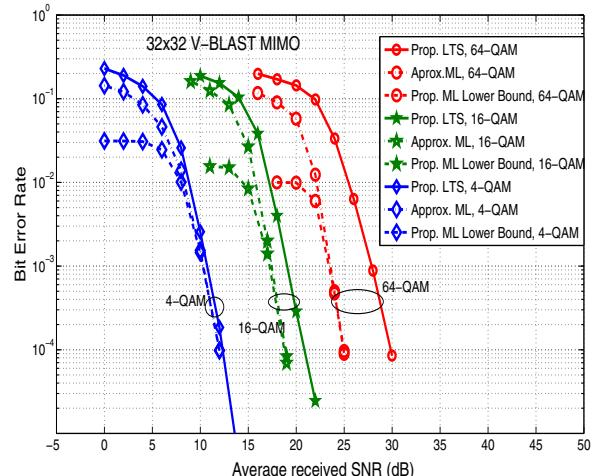
Fig. 6. Performance nearness of LTS with ordering to the proposed lower bound of ML and the approximate ML for  $32 \times 32$  V-BLAST MIMO with 4-, 16-, and 64-QAM.  $n = 1$  for the ML lower bound.
