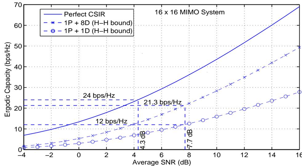
**Figure 4:** H-H capacity bound [13] for 1P+8D ( $T = 144, \tau = 16, \beta_p = \beta_d = 1$ ) and 1P+1D ( $T = 32, \tau = 16, \beta_p = \beta_d = 1$ ) training for a  $16 \times 16$  MIMO channel.
