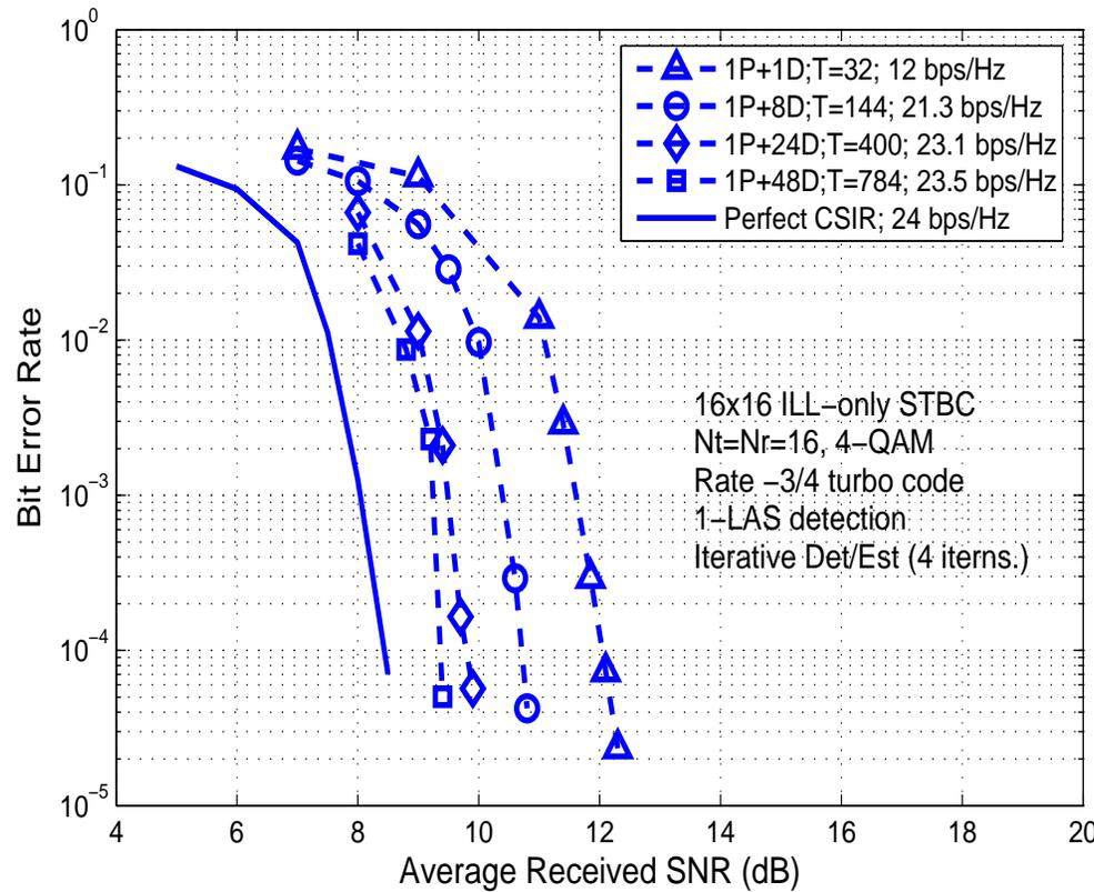
**Figur6:** Turbo coded BER performance of LAS detection and channel estimation as a function of coherence time,  $T = 32, 144, 400, 784$  ( $N_d = 1, 8, 24, 48$ ), for a given  $N_t = N_r = 16$ .  $16 \times 16$  ILL-only STBC, 4-QAM, rate-3/4 turbo code. **Spectral efficiency and BER performance with estimated CSIR approaches to those with perfect CSIR in slow fading (i.e., large  $T$ ).**
