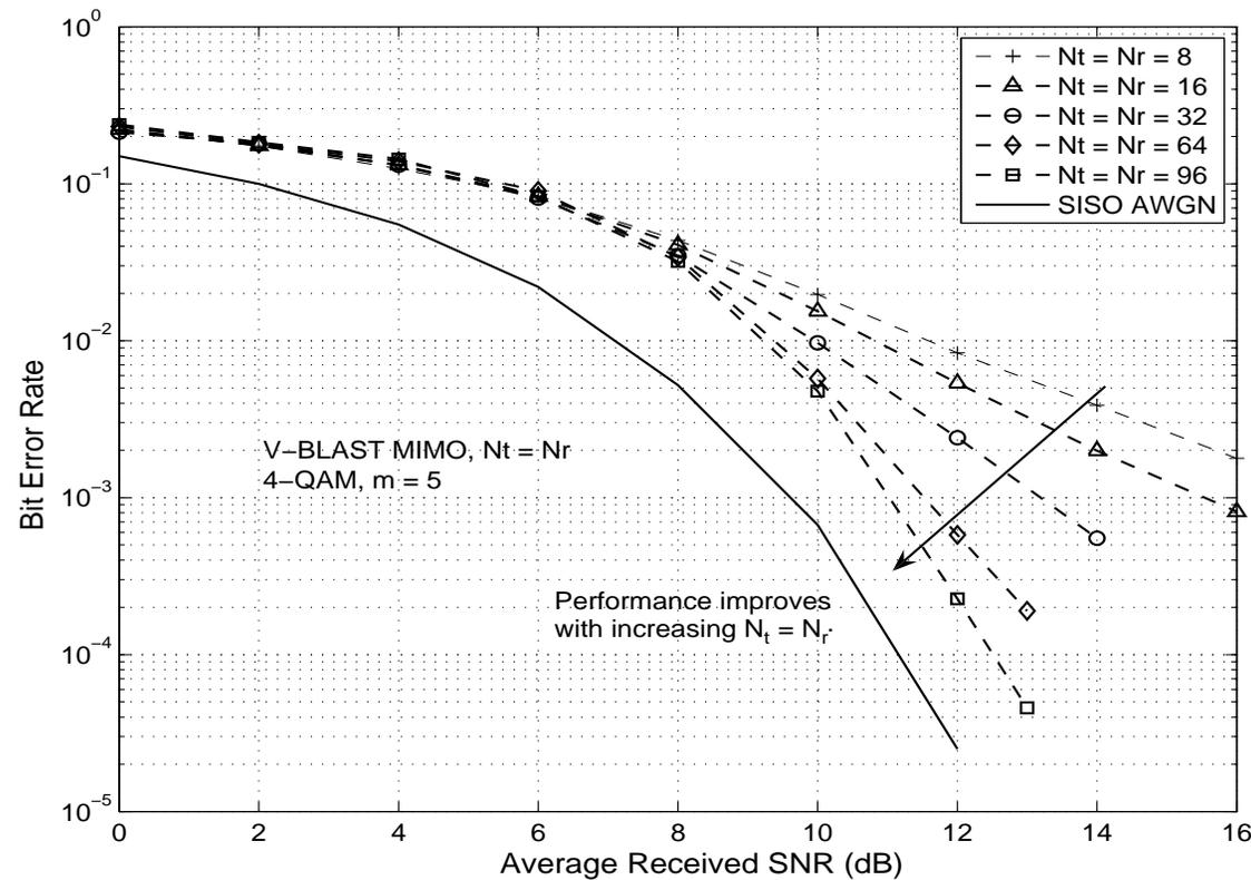
**Figure:** BER performance of PDA based detection of V-BLAST MIMO for  $N_t = N_r = 8, 16, 32, 64, 96$ , 4-QAM, and  $m = 5$  iterations.
