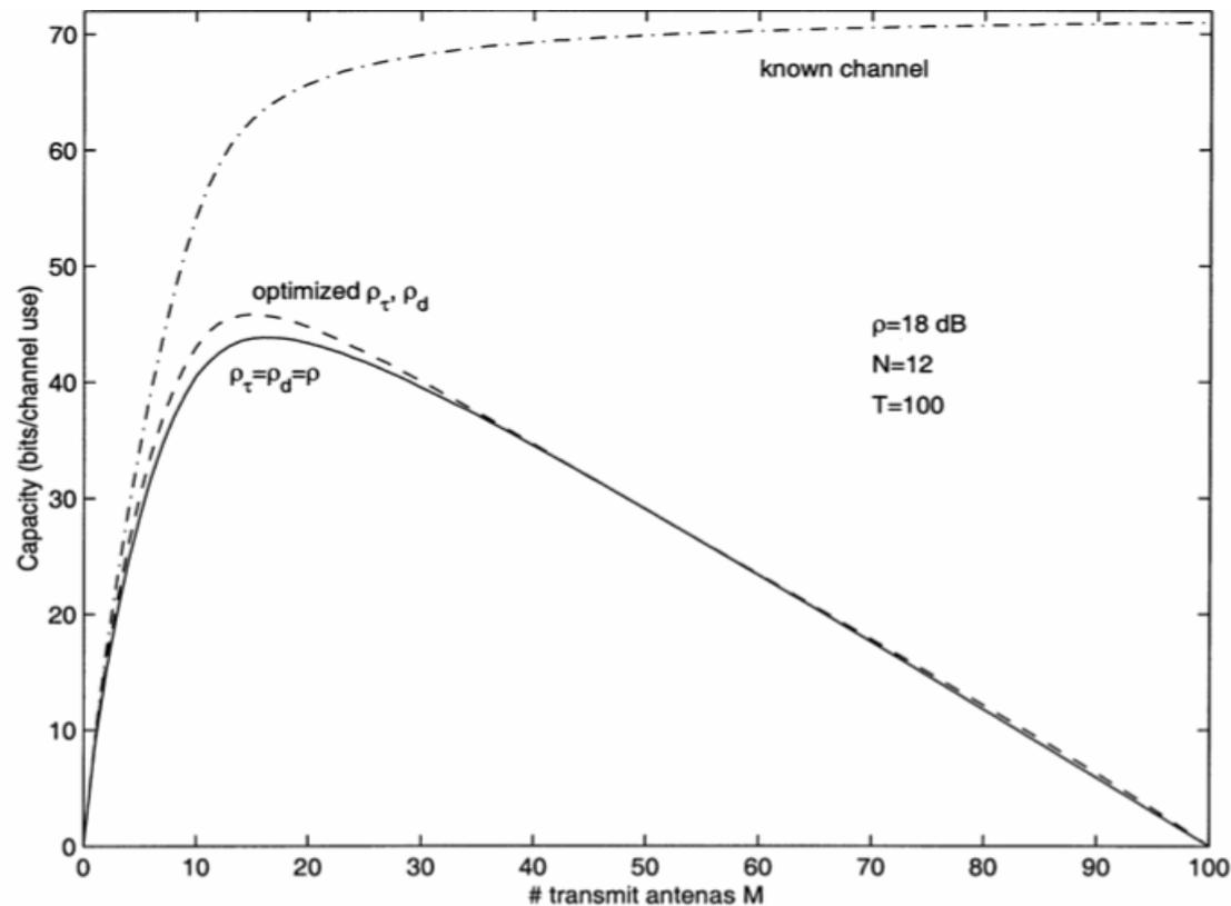
Fig. 5. Capacity as a function of number of transmit antennas  $M$  with  $\rho = 18$  dB and  $N = 12$  receive antennas. The solid line is optimized over  $T_t$  for  $\rho_t = \rho_d = \rho$  (see (40)), and the dashed line is optimized over the power allocation with  $T_t = M$  (Theorem 3). The dash-dotted line is the capacity when the receiver knows the channel perfectly. The maximum throughput is attained at  $M \approx 15$ .
