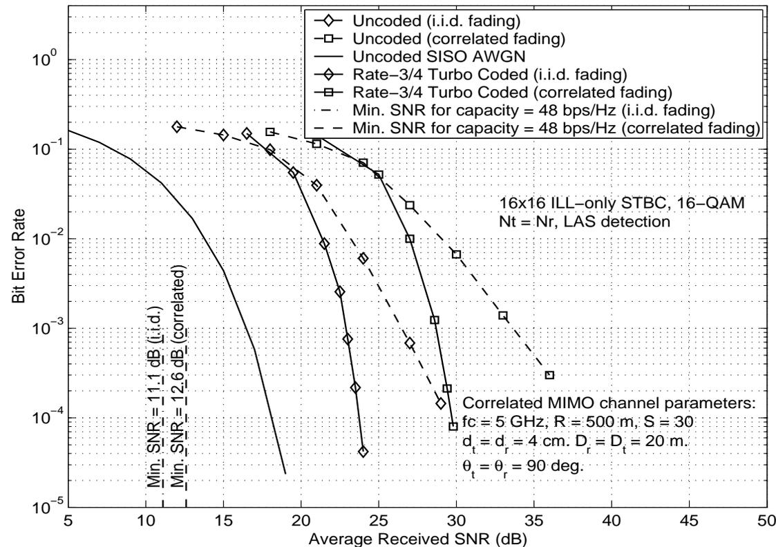
**Figure 2:** Uncoded/coded BER performance of 1-LAS detector *i*) in i.i.d. fading, and *ii*) in correlated MIMO fading in [3] with  $f_c = 5$  GHz,  $R = 500$  m,  $S = 30$ ,  $D_t = D_r = 20$  m,  $\theta_t = \theta_r = 90^\circ$ , and  $d_t = d_r = 2\lambda/3 = 4$  cm.  $16 \times 16$  STBC,  $N_t = N_r = 16$ , 16-QAM, rate-3/4 turbo code, 48 bps/Hz.
