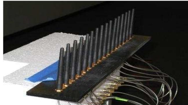
16 Linear Dipole Antenna Array
