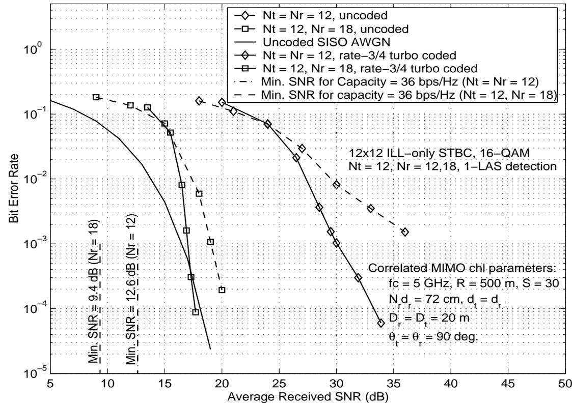
**Figure 8:** Effect of  $N_r > N_t$  in correlated MIMO fading in [3] keeping  $N_r d_r$  constant and  $d_t = d_r$ .  $N_r d_r = 72$  cm,  $f_c = 5$  GHz,  $R = 500$  m,  $S = 30$ ,  $D_t = D_r = 20$  m,  $\theta_t = \theta_r = 90^\circ$ ,  $12 \times 12$  ILL-only STBC,  $N_t = 12, N_r = 12, 18$ , 16-QAM, rate-3/4 turbo code, 36 bps/Hz. **Increasing # receive dimensions alleviates the loss due to spatial correlation.**
