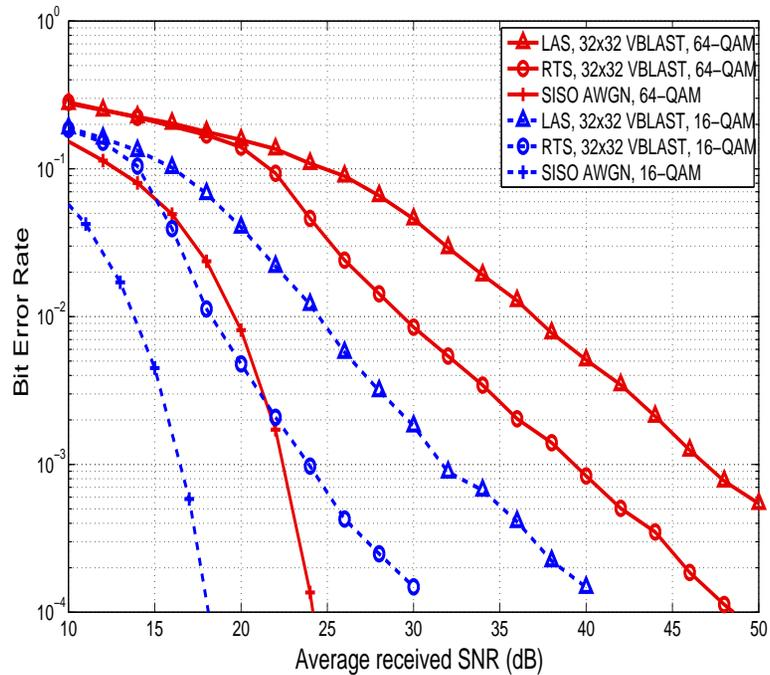
(c) Performance in  $32 \times 32$  V-BLAST,  $M$ -QAM
