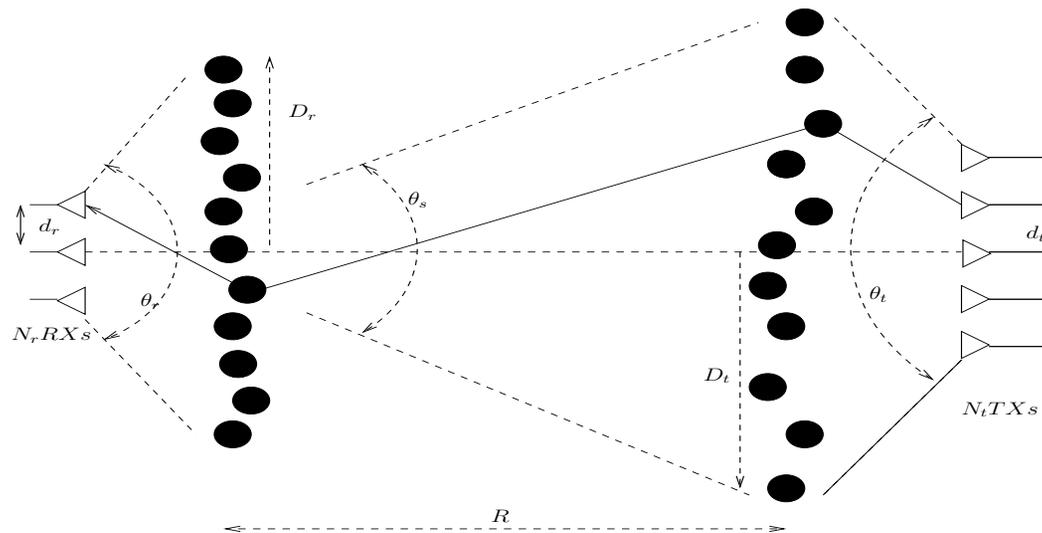
**Figure:** Propagation scenario for the MIMO fading channel model
