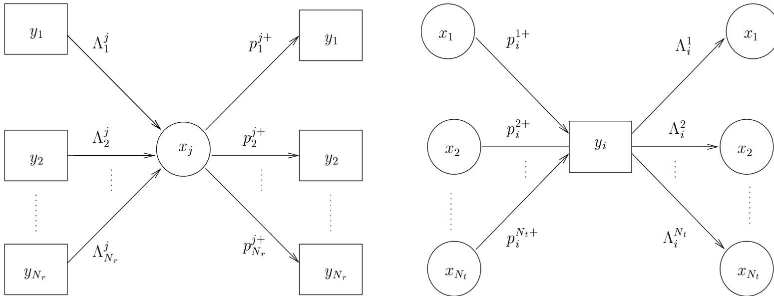
**Figure 8:** Message passing between variable nodes and observation nodes.
