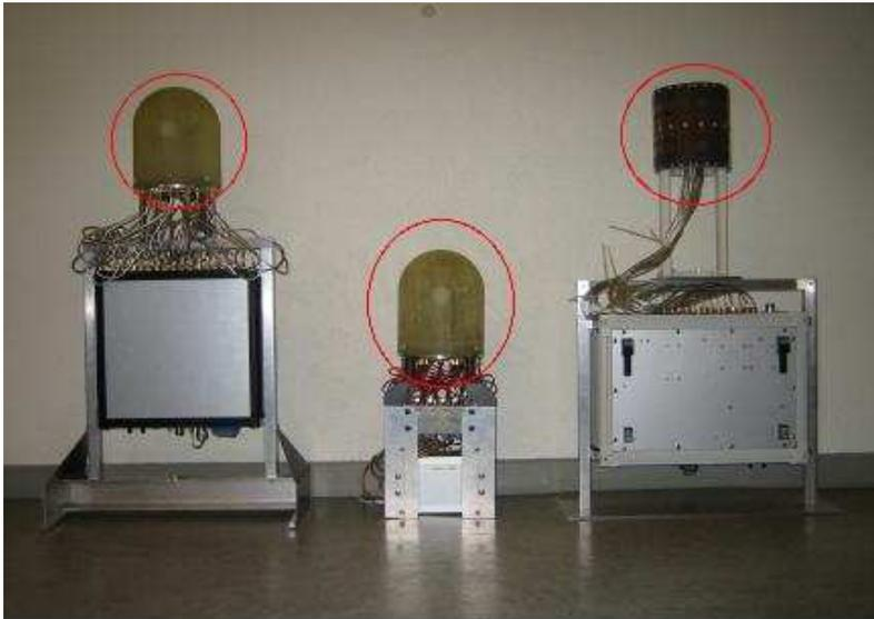
(a) 64-Antenna/RF hardware at 5 GHz
