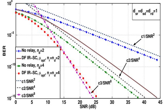
Fig. 4. BER versus SNR plots for SSK in DF IR-SC at optimum threshold values ( $\mu_{opt}$ ) for  $n_r = n_d = 2, 4$ ;  $d_{sr} = d_{sd} = d_{rd} = 1$ . Analysis.
