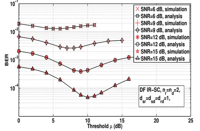
Fig. 3. BER versus  $\mu$  plots for SSK in DF IR-SC cooperative relaying scheme for  $n_r = n_d = 2$ ,  $d_{sr} = d_{sd} = d_{rd} = 1$  for different SNR values (SNR = 6 dB, 9 dB, 12 dB, and 15 dB). Analysis and simulation.
