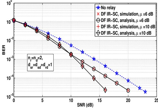
Fig. 2. BER of SSK in DF IR-SC cooperative relaying scheme for  $n_r = n_d = 2$ ,  $d_{sr} = d_{sd} = d_{rd} = 1$  for different threshold values ( $\mu = 6$  dB, 10 dB). Analysis and simulation.
