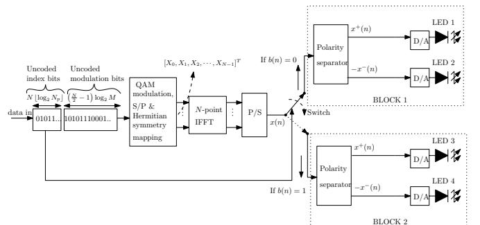
Fig. 2. Proposed I-NDC OFDM transmitter.
