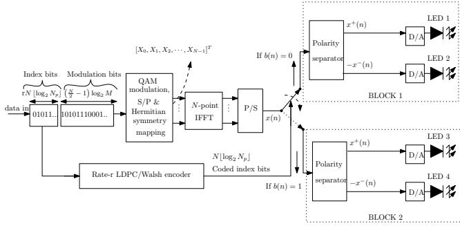
Fig. 7. Proposed CI-NDC OFDM transmitter.
