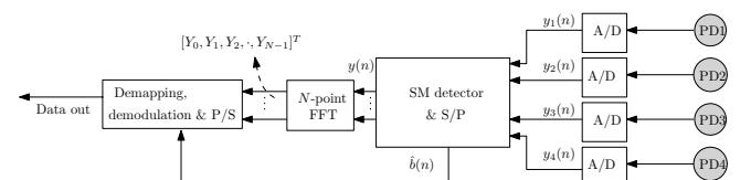
Fig. 3. Proposed I-NDC OFDM receiver.
