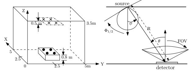
Fig. 4. Geometric set-up of the considered indoor VLC system. A dot represents a photo detector and a cross represents an LED.
