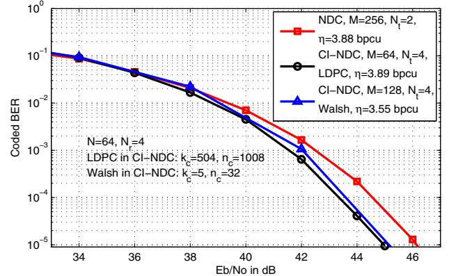
Fig. 9. BER performance of the proposed CI-NDC OFDM and NDC OFDM at  $\eta = 3.8$  bpcu,  $N_r = 4$ .
