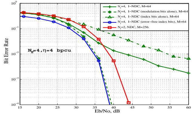
Fig. 6. Reliability of modulation bits and index bits in the proposed I-NDC OFDM for  $\eta = 4$  bpcu,  $N_r = 4$ .
