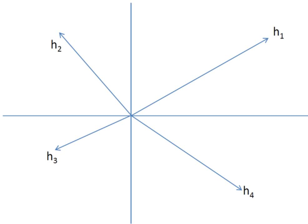
Figure: Effective channel gains in conventional SM
