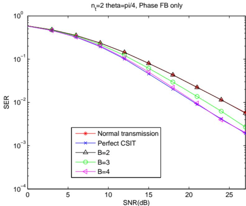
Figure: Comparison of SER for different FB rates
