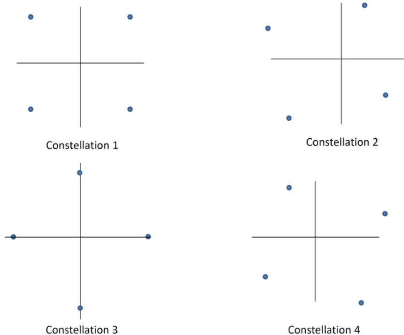
Figure: 4 rotated constellations of QPSK
