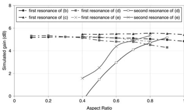
**Figure 5** Variation in the boresight gain of MSR geometries of Fig. 3
