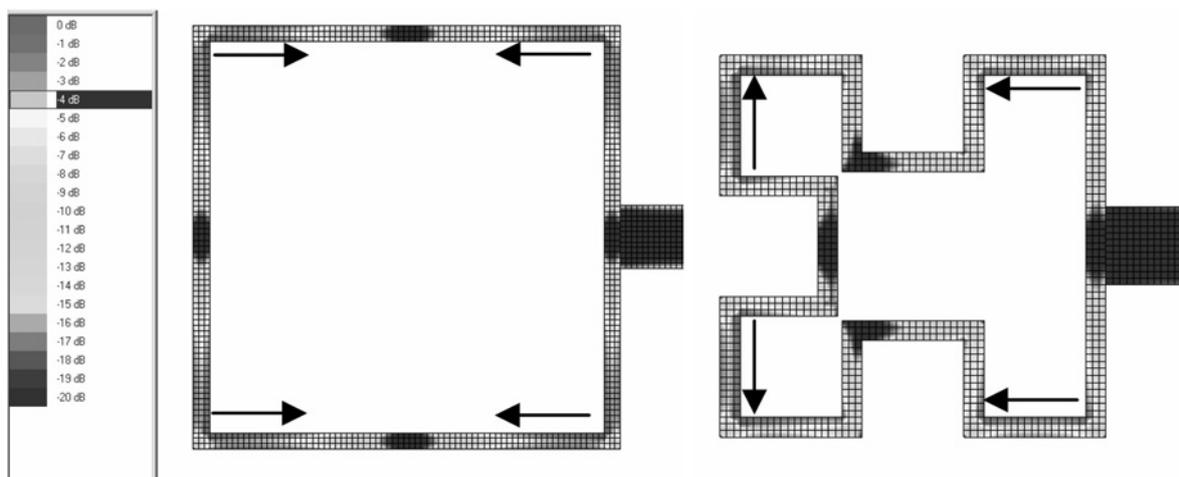
**Figure 6** Average current distribution of antenna geometries by simulations
