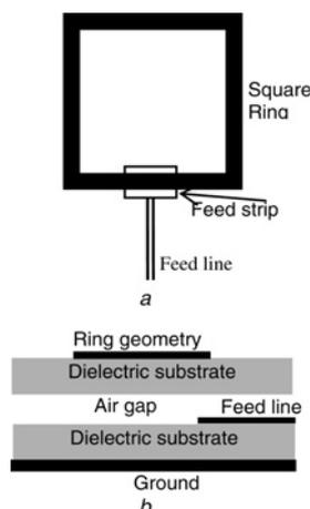
**Figure 1** Schematic of the square ring antenna configuration
