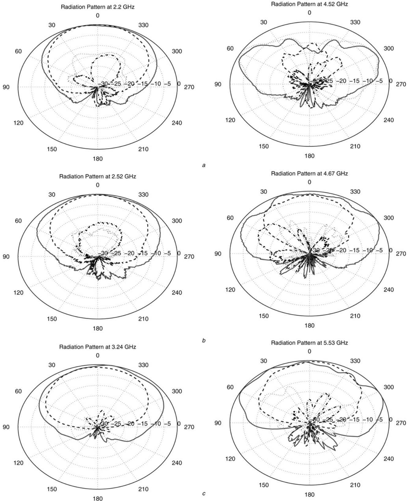
**Figure 8** Measured radiation patterns in E (co: solid, cross: dash-dot) and H (co: dashed, cross: dot-dot) planes at the first and second resonant frequencies of fabricated antennas
