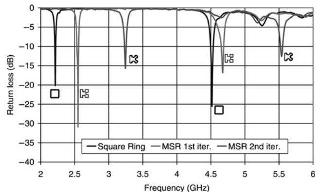
**Figure 7** Measured return loss of the square ring and MSR geometries with aspect ratio of 0.8
