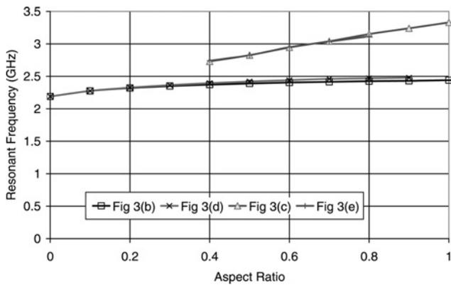
**Figure 4** Primary resonant frequency of various antenna geometries in Fig. 3 as the aspect ratio of the fractal geometry is varied
