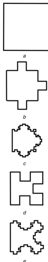
**Figure 3** Minkowski-square ring with sides replaced by fractal geometry on one, two and three sides at first and second iteration
