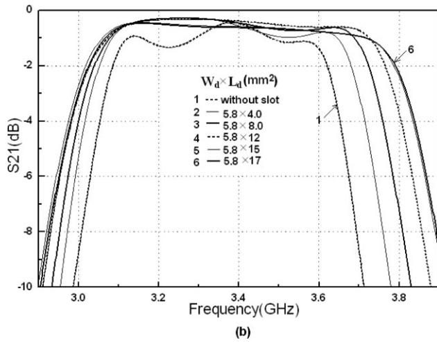
**Figure 5** Effect of slot in bottom ground plane on bandwidth: (a) Change in width 'W<sub>d</sub>'; (b) Change in length 'L<sub>d</sub>'
