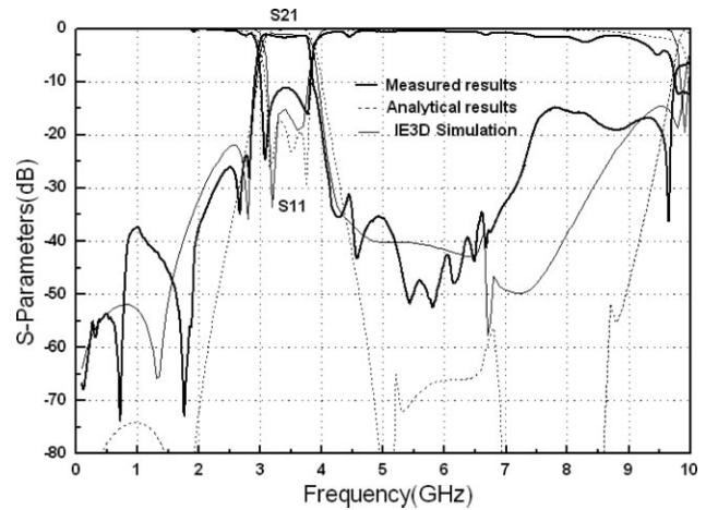
**Figure 8** Measured results of wideband bandpass filter
