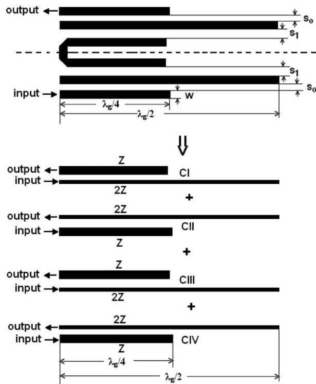
Figure 3 Coupled line sections in Layer 1 and their equivalence
