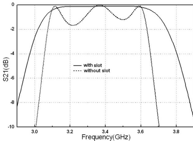
**Figure 6** Analytical results of filter with and without slot in the bottom ground plane
