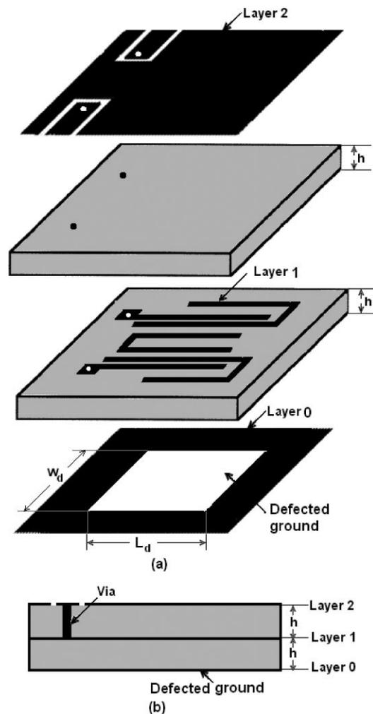
**Figure 1** Wide bandpass filter. (a) Exploded view of different layers. (b) Cross sectional view of the complete device
