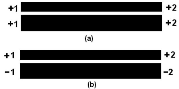
Figure 4 Coupled line excitations for EM simulation
