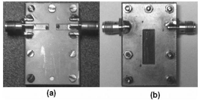
**Figure 7** Photograph of assembled wideband bandpass filter: (a) Top view; (b) Bottom view
