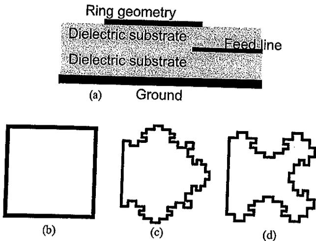
Fig.5. Square ring antenna (a) cross sectional view and (b)-(d) Top views: (b) square geometry (c) and (d) two approaches of replacing straight segments with second iteration fractal Minkowski curves
