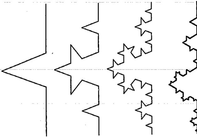
Fig.3. Various geometries of Koch curves (a) iteration 1, (b) iteration 2, (c) iteration 3, and (d) 3rd iteration geometry without self-similarity
