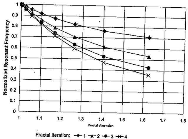
Fig.2. The normalized resonant frequency of generalized Koch dipole antennas of different fractal iterations
