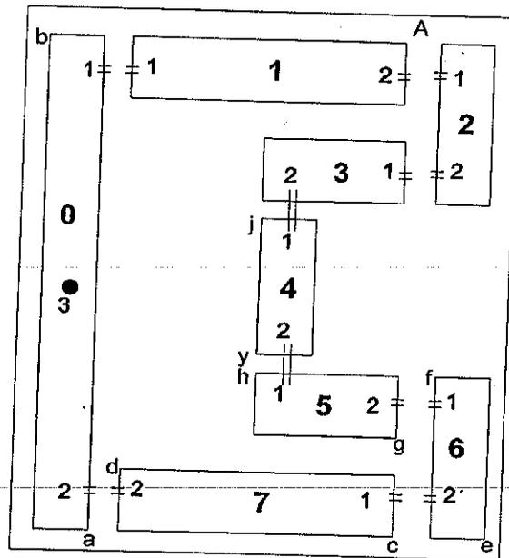
Fig.7 Segmentation of Square ring microstrip antenna with one side replaced by fractal geometry at first iteration
