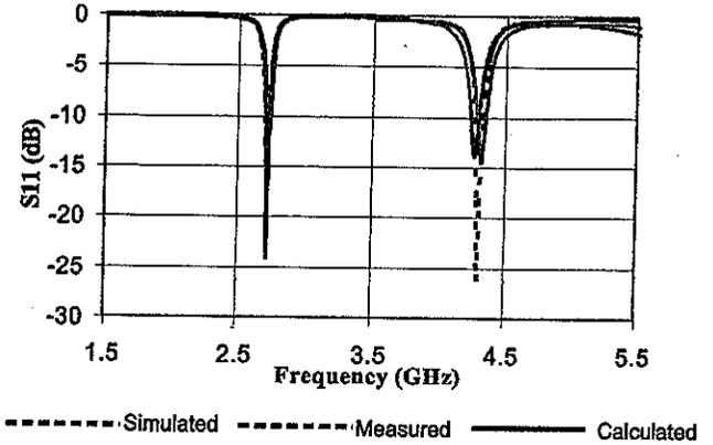
Fig.8 Return loss characteristics of the Fractal Microstrip ring antenna shown in Fig.6
