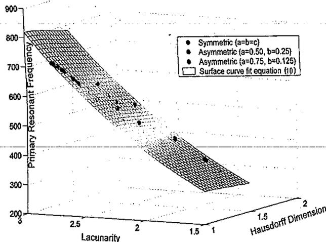
Fig.4. Resonant frequency of Koch dipole antennas calculated with Eq. (10) and numerical simulations
