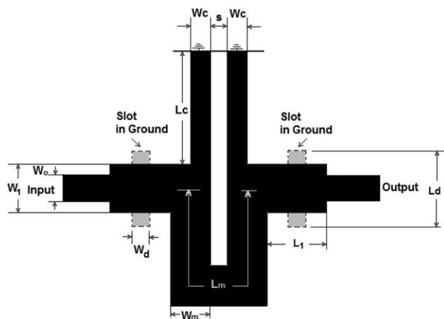
Figure 1 Extended stop band UWB filter
