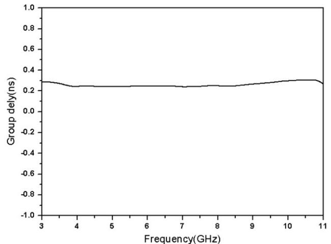
Figure 8 Measured group delay
