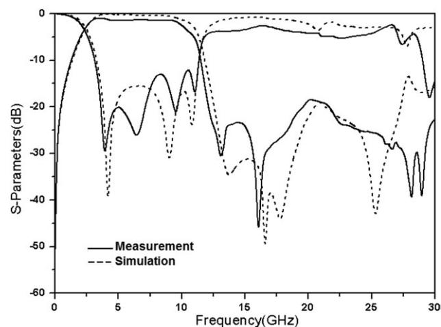
Figure 7 Measured results of UWB filter
