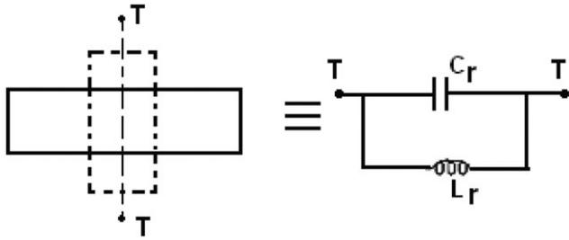
Figure 3 DGS and its equivalent
