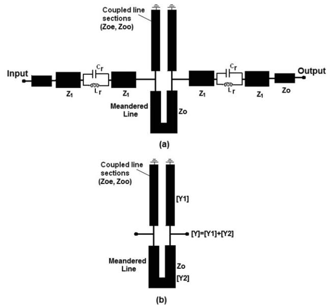
Figure 2 (a) Circuit model of the filter and (b) circuit model of the embedded coupled line section
