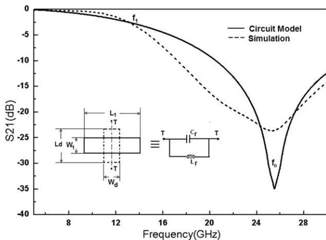
Figure 4 Response of line with DGS
