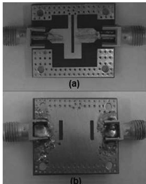
Figure 6 Photograph of the assembled UWB filter
