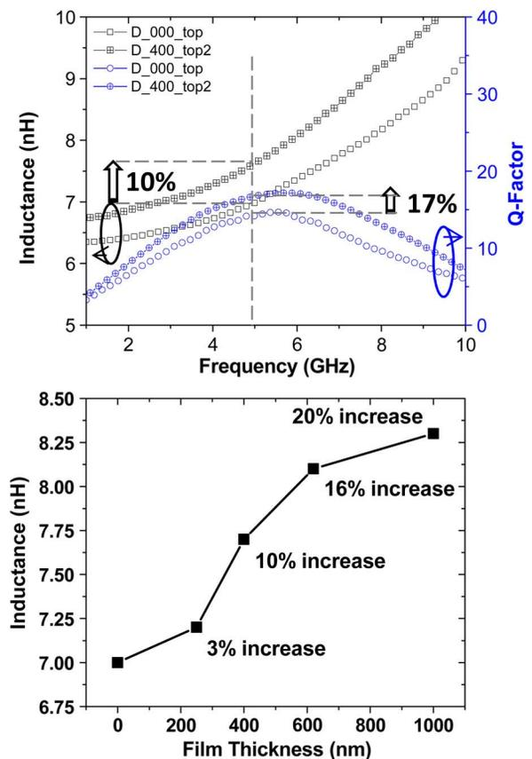
Fig. 6. (top) Frequency-dependent plot of inductance and Q-factor of the on-chip RF spiral inductor with ZFTF of 400 nm deposited on top, yielding a 10% enhancement of inductance at 5 GHz; (bottom) Plot shows the increase of inductance and thus inductance density with various thickness of ZFTF deposited on top of the inductor.
