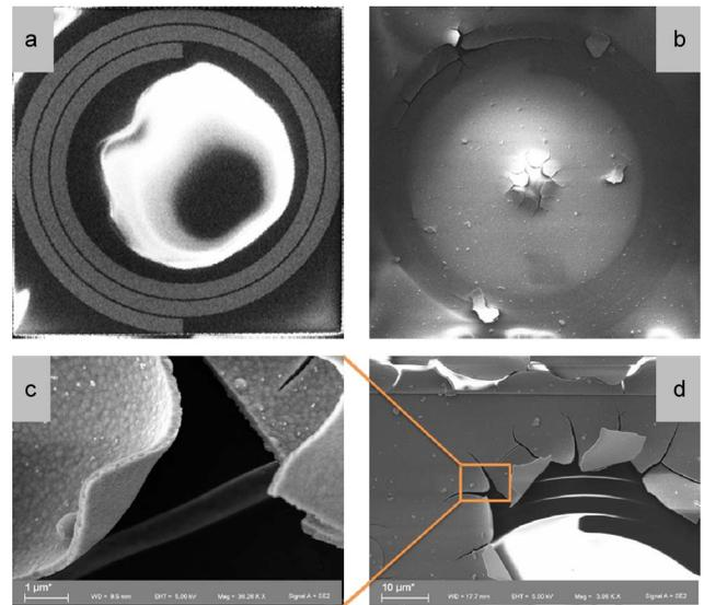
Fig. 5. SEM image of the inductor structure (a) before deposition; (b) after deposition; (c) and (d) demonstrating the morphology and the uniformity of the film deposited on the inductor structure. (The film was deliberately peeled-off for characterization).
