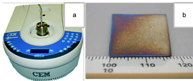
Fig. 1. (a) Single-mode microwave reactor. (b) Optical micrograph of the deposited zinc ferrite film on a Si (100), illustrating uniformity and large area coating capability.
