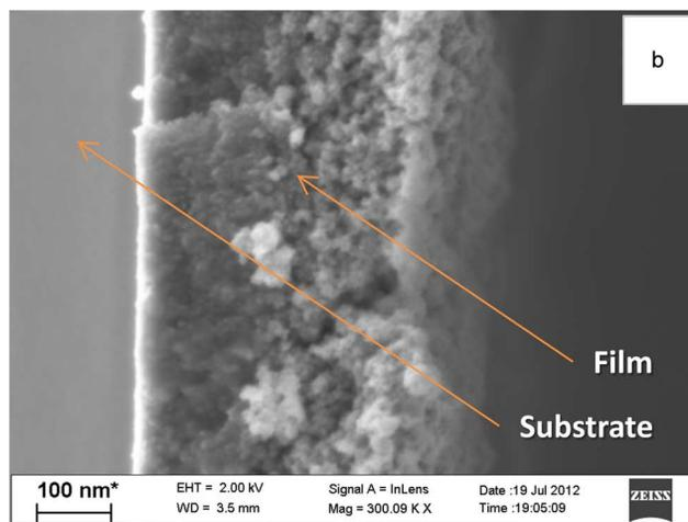
Fig. 2. (a) XRD pattern of the ZFTF. (b) Cross-sectional SEM image of a 400 nm-thick ZFTF, revealing the presence of very small ( $< \sim 5$  nm) crystallites.
