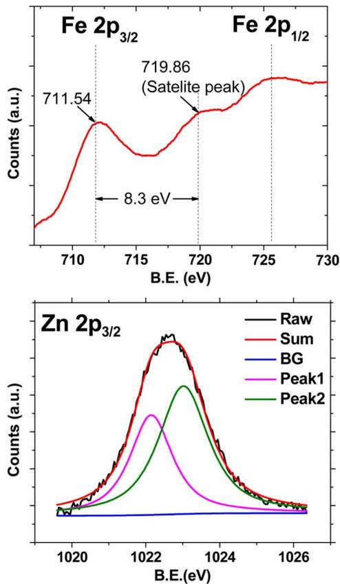
Fig. 3. X-ray photoelectron spectra of (a) Fe 2p and (b) Zn  $2p_{3/2}$ . In Fe 2p spectra presence of satellite peak confirms the absence of  $\text{Fe}^{2+}$  and the splitting of Zn  $2p_{3/2}$  confirms the partially inverted structure of the ZFTF.
