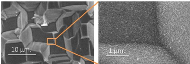
Fig. 4. SEM micrograph of ZFTF the deposited on the back side of the Si (100) substrate, demonstrating the conformal nature of the deposition process.
