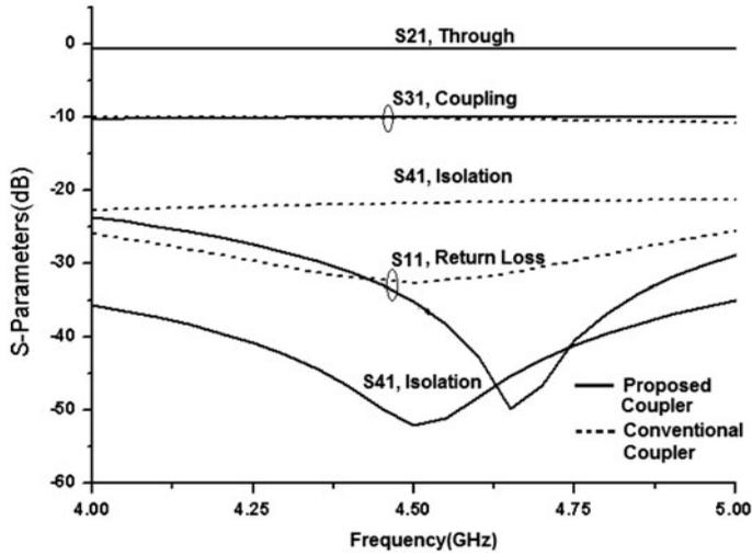
Figure 4. Simulation results of the proposed coupler.
