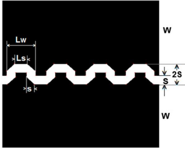
Figure 3. Dimensions of wiggly structure (top layer).
