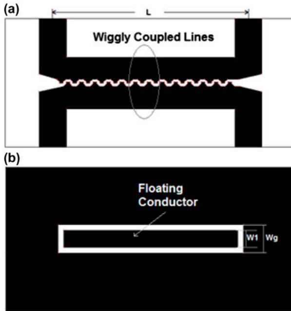
Figure 2. The proposed high directivity coupler. (a) Top layer, (b) bottom layer.
