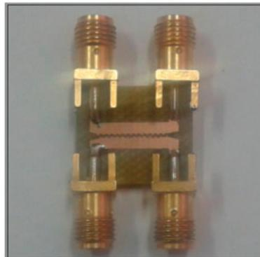
Figure 6. Assembled high directivity coupler.
