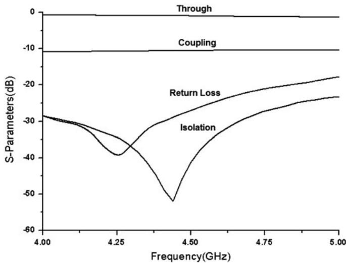
Figure 8. Measured characteristics of high directivity coupler.
