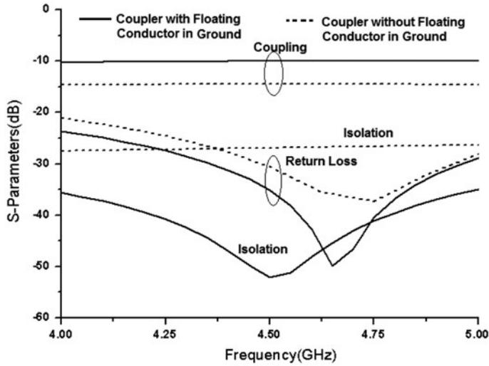
Figure 5. Simulation performance of proposed coupler with and without floating conductor in the ground.
