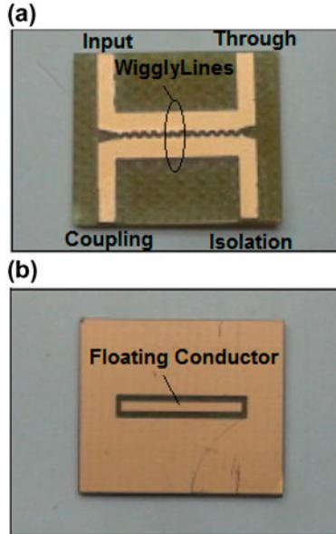
Figure 7. Layers of coupler. (a) Top, (b) bottom.
