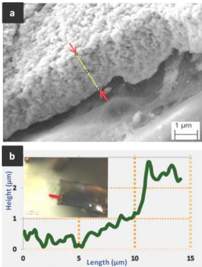
Fig. 4. Thickness of electrodeposited copper film. (a) Cross-section FESEM image shows that copper nanoparticles have aggregated to form the film. The thickness of the film was estimated to be  $1.8 \mu\text{m}$ . (b) Height profile, using an optical profilometer, along a paper-fiber and across the edge of the copper film (corresponding to the red line in the inset). The average thickness estimated from this profile corresponds well with FESEM measurements.
