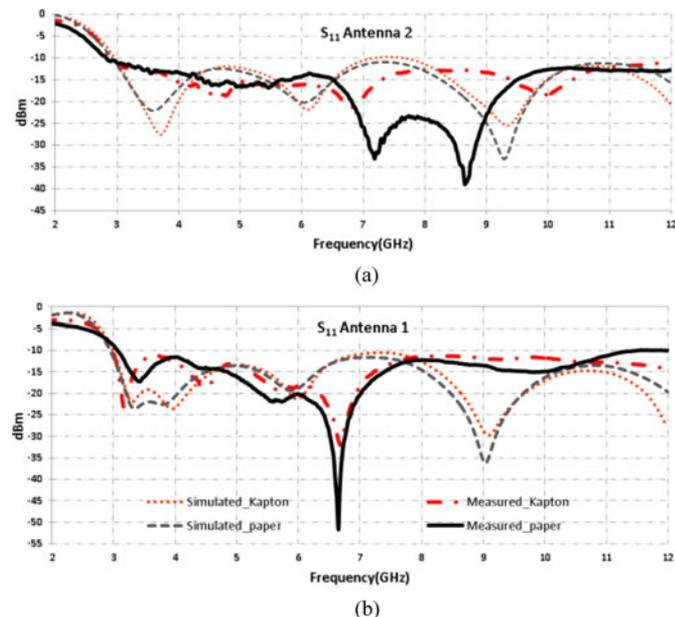
Fig. 5. Measured transfer characteristics ( $S_{11}$ ) of fabricated antennas. (a) Antenna 2 and (b) Antenna 1. The  $-10\text{-dB}$  bandwidth of both antennas on paper span from 3 to 11 GHz, covering the entire UWB spectrum. The performance of paper and Kapton-based antennas are comparable.
