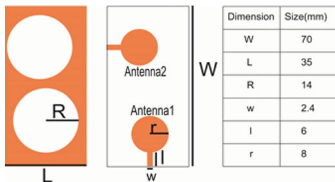
Fig. 1. Design layout of the fabricated antenna structures along with antenna dimensions.
