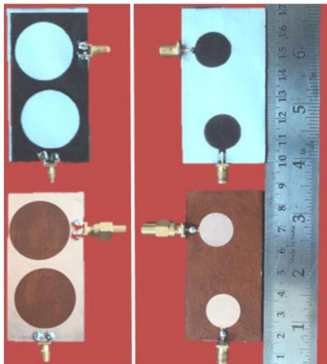
Fig. 2. Digital photographs of the two sides of UWB antennas fabricated on paper (top) by using reactive inkjet printing and electroless deposition, and on Kapton (bottom) by using lithographic processes. The electrodeposited copper has a much rougher microstructure and appears black in color, while the copper cladding on Kapton has a lustrous metallic sheen.
