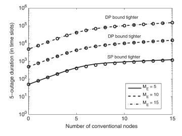
Fig. 2. 5-outage duration as a function of  $M_C$  for different  $M_E$  ( $\rho = 0.5$ ,  $E_{tx}/E_h = 3$ , and  $\gamma_{th} = 1$ ). Simulation results are shown using the marker  $\circ$ . The lines depict the bound in (13).
