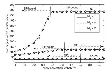
Fig. 5. 5-outage duration as a function of energy harvesting probability ( $M_C = 3$ ,  $E_{tx}/E_h = 3$ , and  $\gamma_{th} = 1$ ). Simulation results are shown using the marker  $\circ$ . The lines depict the bound in (13).
