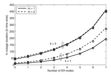
Fig. 4. Effect of k and channel fading statistics on the k-outage duration  $(M_C = 5, \rho = 0.1, E_{\rm tx}/E_h = 1, \text{ and } \gamma_{\rm th} = 1)$ . Simulation results are shown using the marker  $\circ$ . The lines depict the bound in (13).
