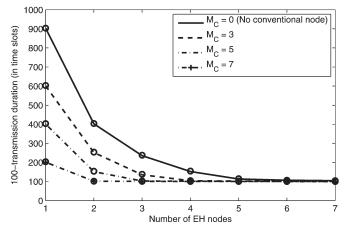
Fig. 6. 100-transmission duration as a function of  $M_E$  for different  $M_C$  ( $\rho = 0.1, E_{\rm tx}/E_h = 1$ , and  $\gamma_{\rm th} = 1$ ). Simulation results are shown using the marker  $\circ$ . The lines depict the bound in (21).
