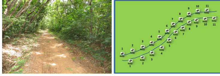
Fig. 4. A segment of the trail in the Jubilee Gardens in the Indian Institute of Science campus. Motes were mounted on trees along each side of the trail at a height of about 2 meters. The right panel shows a depiction of the deployment of 22 motes along a stretch of the trail. Several network deployments were made with this setup. All the nodes in each such network were among nodes 1, 2, \dots , 11 on one side of the trail (say, the “left” side) or nodes 1, 2, \dots , 11 on the right side of the trail (say, the “right” side). Thus, radio propagation was always “through” the foliage.
