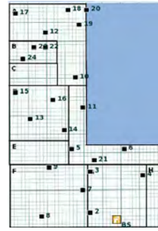
Fig. 12. Set of 24 locations where nodes were placed and link learning performed periodically to evaluate network robustness
