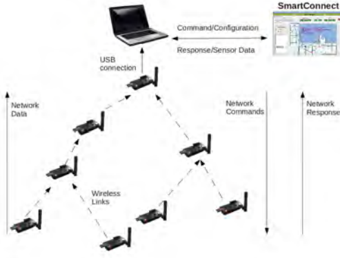
Fig. 6. SmartConnect architecture: Iterative deployment involves command-response interaction between nodes on the field and the SmartConnect system via the SmartConnect-WSN gateway; message interaction between the SmartConnect graphical user interface (GUI) and SmartConnect-WSN gateway takes place over TCP/IP.
