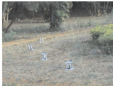
Figure 14: Three sensors platform and the wireless trip-wire.
