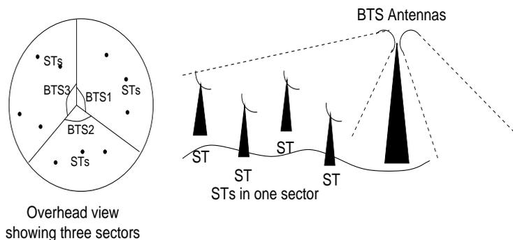
Fig. 1. WiFiRe network configuration. The figure on the left shows a deployment with three sectors, and the figure to the right shows a tall tower carrying several BSs, with sector antennas, and several STs in a sector, with lower height directional antennas.
