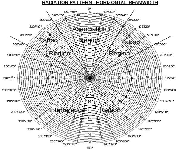
Fig. 2. Radiation pattern of a typical BS antenna that could be used in the deployment. The association region is a  $60^\circ$  sector centered at the  $0^\circ$  mark, the taboo region is  $30^\circ$  on either side of this association region, and the limited interference region covers the remaining  $240^\circ$ .
