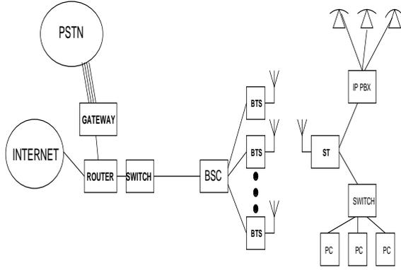
Fig. 3. A possible network access architecture for a Wi-Fi deployment.
