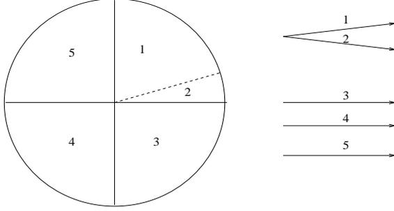
Fig. 7. Deployment of a system with 4 sectors and 5 STs
