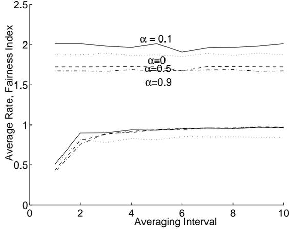
Fig. 8. Variation of total rate and fairness index with averaging interval for different values of  $\alpha$ . The upper set of plots are of the total rate, and bottom set are for the fairness index.
