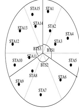
Fig. 6. A typical deployment of a system with 3 sectors and 15 STs.
