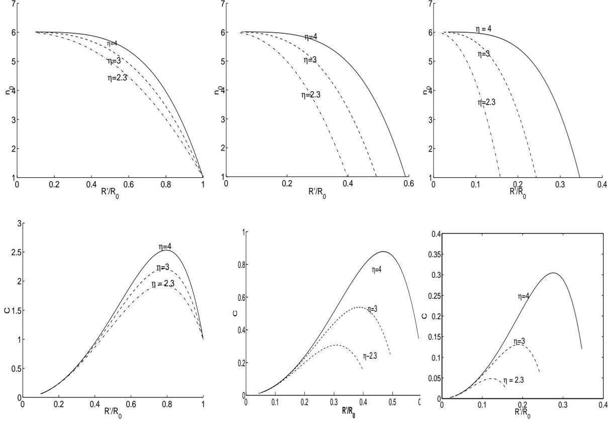
Fig. 4. Variation of the number of simultaneous transmissions possible ( $n_0$ ) and system capacity ( $C$ ) with coverage relative to a reference distance  $R_0$  for  $\eta = 2.3, 3, 4$  and  $\sigma = 0, 4, 8$ . Plots for  $\sigma = 0, 4, 8$  are shown left to right.
