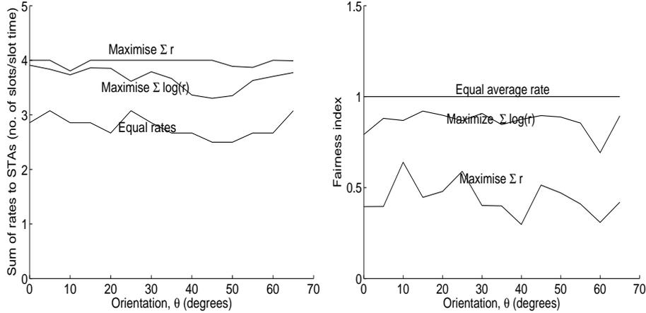
Fig. 5. Variation of sum rate and fairness index with antenna orientation for different utility functions.
