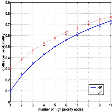
Fig. 13. Plots of collision probability of HP - Priority 0 (AC\_VO) nodes and LP - Priority 2 (AC\_BE) nodes with the number of Priority 2 nodes fixed to 4. The lines correspond to the fixed point analysis, the “+” correspond to the ns-simulations and “o” correspond to the CMP simulator. The 95% confidence interval lies within 1% of the simulation estimate.
