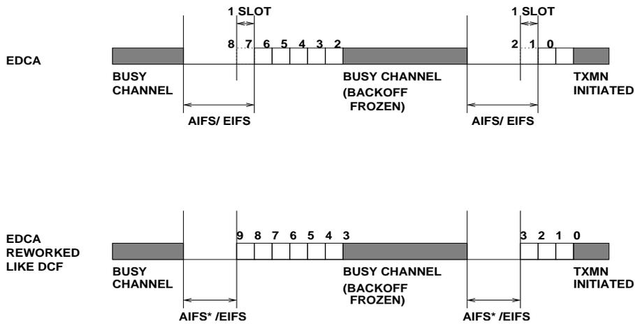
Fig. 3. IEEE 802.11e EDCA backoff compared with a “DCF like” scheme with  $AIFS^* := AIFS - aSlotTime$  and  $BC^* := BC + 1$ , where  $BC = 8$  is the residual backoff counter value. We note that because of the way IEEE 802.11e EDCA decrements backoff,  $[0, CW]$  is actually equivalent to  $[1, CW+1]$  (for AIFS appropriately defined).
