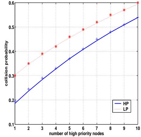
Fig. 15. Plots of collision probability of HP - Priority 1 (AC\_VI) nodes and LP - Priority 2 (AC\_BE) nodes with the number of Priority 2 nodes fixed to 8. The lines correspond to the fixed point analysis and the symbols correspond to the CMP simulator. The 95% confidence interval lies within 1% of the simulation estimate.
