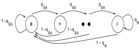
Fig. 12. AIFS differentiation mechanism: Markov model for remaining number of AIFS slots.
