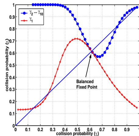
Fig. 2. Example System-I: Demonstration of unbalanced fixed points. Plots of  $\gamma_2 = 1 - (1 - G(\gamma))^8(1 - G(1 - (1 - G(\gamma))^9))$  (the curve drawn with dots and lines) and the function for the fixed point equation for  $\gamma_1$  (see text) using pluses and lines.
