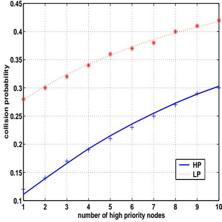
Fig. 17. Plots of collision probability of HP - Priority 2 (AC\_BE) nodes and LP - Priority 3 (AC\_BK) nodes with the number of Priority 3 nodes fixed to 8. The lines correspond to the fixed point analysis and the symbols correspond to the CMP simulator. The 95% confidence interval lies within 1% of the simulation estimate.
