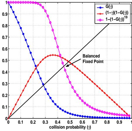
Fig. 5. Example System-II: The balanced fixed point. Plots of  $G(\gamma)$ ,  $F(\gamma) = (1 - \gamma)(1 - G(\gamma))$  and  $1 - (1 - G(\gamma))^{19}$  vs. the collision probability  $\gamma$ ; the line “ $y=x$ ” is also shown. Notice that the function  $F$  is not one-to-one.
