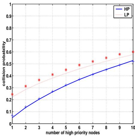
Fig. 16. Plots of collision probability of HP - Priority 1 (AC\_VI) nodes and LP - Priority 3 (AC\_BK) nodes with the number of Priority 3 nodes fixed to 4. The lines correspond to the fixed point analysis and the symbols correspond to the CMP simulator. The 95% confidence interval lies within 1% of the simulation estimate.
