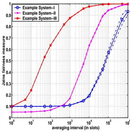
Fig. 10. Throughput fairness index is plotted against the number of slots used to measure throughput. The dotted lines mark the 95% confidence interval.
