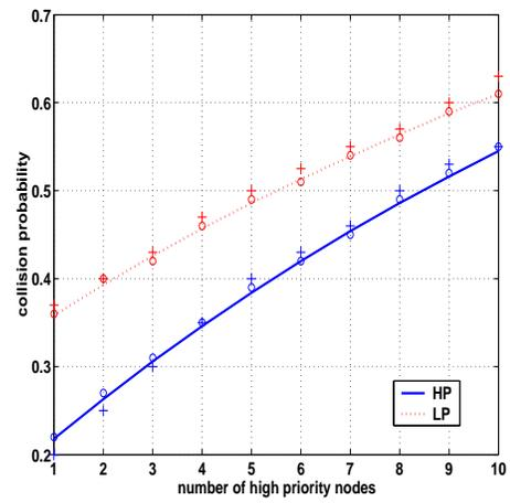
Fig. 14. Plots of collision probability of HP - Priority 1 (AC\_VI) nodes and LP - Priority 2 (AC\_BE) nodes with the number of Priority 2 nodes fixed to 12. The lines correspond to the fixed point analysis, the “+” correspond to the ns-simulations and “o” correspond to the CMP simulator. The 95% confidence interval lies within 1% of the simulation estimate.
