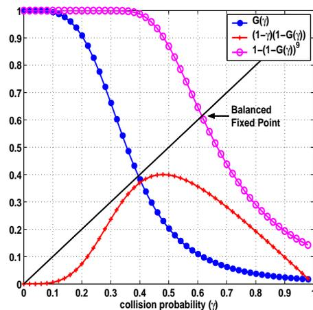
Fig. 1. Example System-I: The balanced fixed point. Plots of  $G(\gamma)$ ,  $F(\gamma) = (1-\gamma)(1-G(\gamma))$  and  $1 - (1 - G(\gamma))^9$  vs. the collision probability  $\gamma$ ; we also show the “ $y=x$ ” line.
