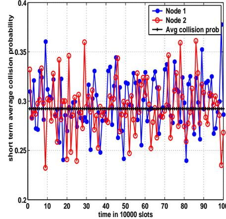
Fig. 9. Example System-III: Snap-shot of short term average collision probability of 2 of the 10 nodes. Also plotted is the average collision probability obtained by the nodes. The 95% confidence interval of the average collision rate lies within 0.2% of the mean value.
