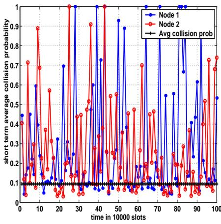
Fig. 7. Example System-II: Snap-shot of short term average collision probability of 2 of the 20 nodes. The average collision probability is also plotted in the figure (averaged over all slots and nodes). The 95% confidence interval for the average collision rate lies within 0.7% of the mean value.
