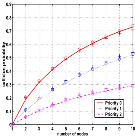
Fig. 11. Plots of collision probability for a homogeneous system of nodes. Three different cases are considered, Priority 0 (AC\_VO), Priority 1 (AC\_VI) and Priority 2 (AC\_BE). The lines correspond to the fixed point analysis, the “+” correspond to the ns-simulations and “O” correspond to the CMP simulator. The 95% confidence interval lies within 1% of the simulation estimate.
