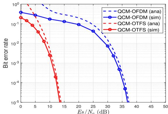
Fig. 5: BER performance of QCM-OTFS ( $M = 2$ ,  $N = 4$ , BPSK, 1 bpcu) and QCM-OFDM ( $M = 8$ , BPSK, 1 bpcu) with Rx located at (2,3).
