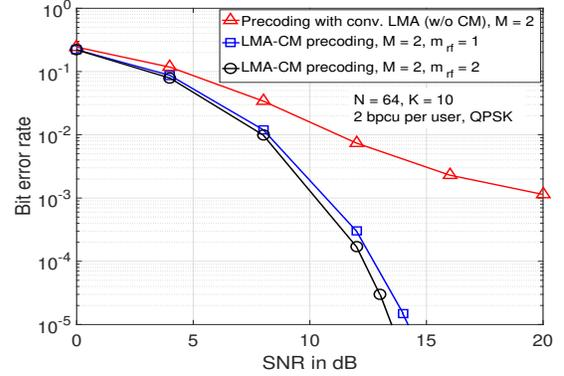
Fig. 5. BER performance of the proposed LMA-CM precoding scheme with  $N = 64$ ,  $K = 10$ ,  $M = 2$ ,  $m_{rf} = 1, 2$ , QPSK, and the proposed iterative algorithm. Performance of precoding with conventional LMA with  $M = 2$  is also shown.
