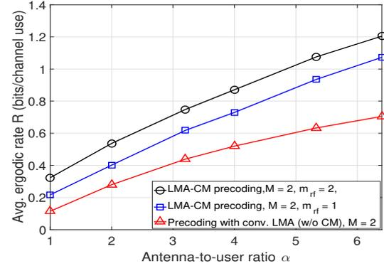
Fig. 4. Lower bound on the average ergodic rate of the proposed LMA-CM precoder with  $M = 2$ ,  $m_{r,f} = 1, 2$ , and the proposed iterative algorithm.
