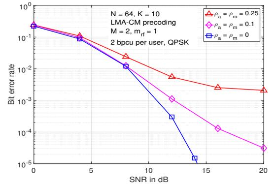
Fig. 6. BER performance of the proposed LMA-CM precoding scheme with  $N = 64$ ,  $K = 10$ ,  $M = 2$ ,  $m_{rf} = 1$ , QPSK, and the proposed iterative algorithm in the presence of spatial correlation.
