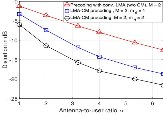
Fig. 2. Distortion versus antenna-to-user ratio for the proposed LMA-CM precoding scheme with  $N = 64$ ,  $m_{r,f} = 1, 2$ ,  $M = 2$ , and proposed iterative algorithm. Performance of precoding with conventional LMA with  $M = 2$  is also shown.
