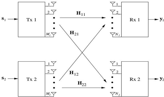
Fig. 1. MIMO X channel system model.
