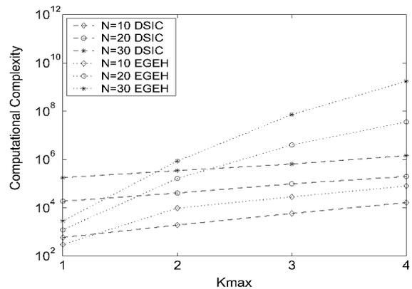
Fig. 10. Computational complexity versus  $K_{max}$  obtained from simulations.  $N = 10, 20, 30$ , number of targets,  $M = 4$ .
