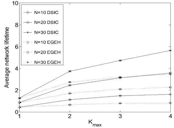
Fig. 5. Average network lifetime versus  $K_{max}$  for  $N = 10, 20, 30, M = 1, \alpha = 1, \epsilon = 0.683, R = 1, E_0 = 2J$
