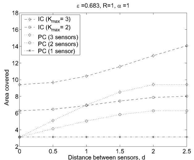
Fig. 4. Area covered by physical coverage (PC) and information coverage (IC).  $\alpha = 1$ ,  $R = 1$ ,  $\epsilon = 0.683$ .
