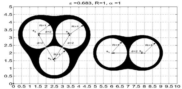
Fig. 3. Illustration of area covered by physical coverage and information coverage.
