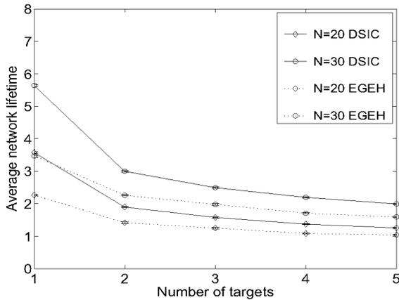
Fig. 8. Average network lifetime versus number of targets,  $M$ , to monitor.  $N = 30, 20$ ,  $K_{max} = 4$ ,  $\alpha = 1$ ,  $\epsilon = 0.683$ ,  $R = 1$ ,  $E_0 = 2 J$ .
