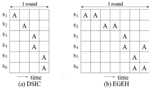
Fig. 7. Illustration of scheduling of sensor activity in DSIC and EGEH.
