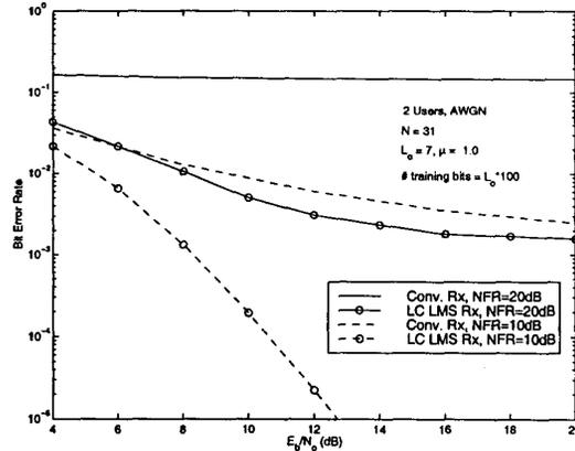
Figure 3: BER performance of Long Code LMS vs Conventional receiver on AWGN channel.  $N = 31$ .  $L_o = 7$ . # training bits =  $L_o * 100$ .
