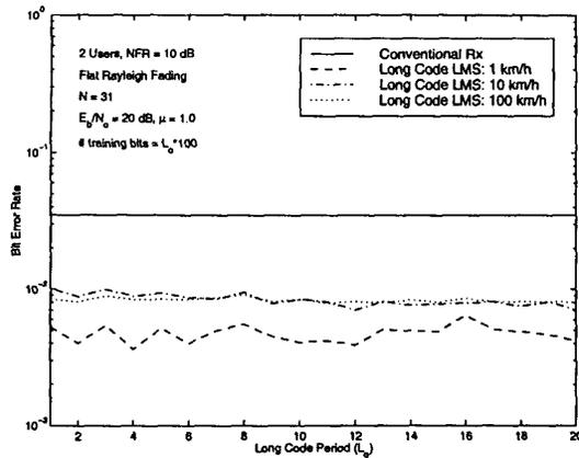
Figure 6: Performance of LC-LMS Rx as a function of  $L_o$ . Rayleigh fading at different user speeds.  $N = 31$ .  $E_b/N_o = 20$  dB.  $NFR = 10$  dB. # training bits =  $L_o * 100$ .
