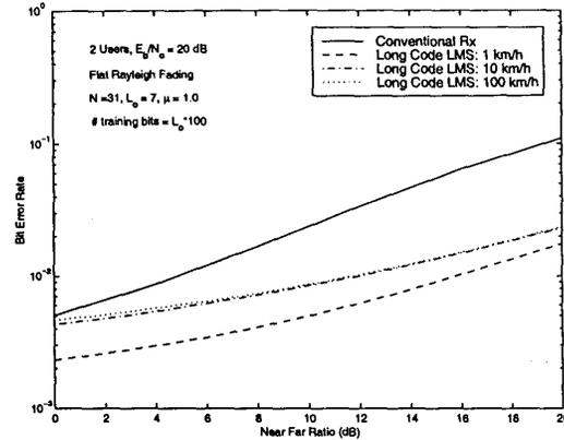
Figure 5: Performance of LC-LMS Rx as a function of NFR. Rayleigh fading.  $N = 31$ .  $E_b/N_o = 20$  dB.  $L_o = 7$ . # training bits =  $L_o \cdot 100$ .
