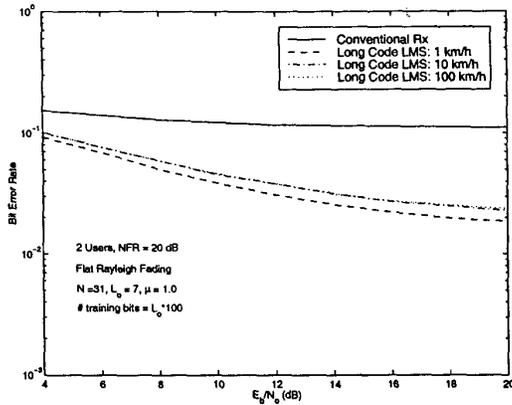
Figure 4: Performance of LC-LMS *vs* Conventional Rx on Rayleigh fading at different user speeds.  $N = 31$ .  $NFR = 20$  dB.  $L_o = 7$ . # training bits =  $L_o \cdot 100$ .
