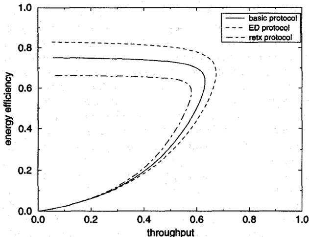
Fig. 1. Energy efficiency vs throughput for various protocols in *slow fading*, i.e.,  $f_{DT} = 0.02$ .  $N = 10$ .  $g_d = 0.1$ .  $b \rightarrow \infty$ .  $F = 5$  dB.
