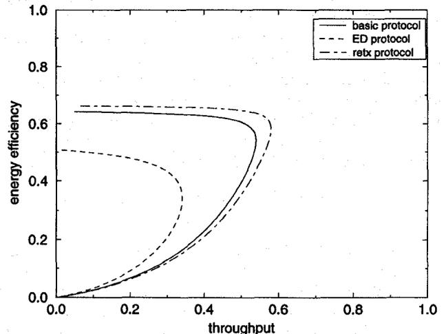
Fig. 2. Energy efficiency vs throughput for various protocols in *fast fading*, i.e.,  $f_{DT} = 0.64$ .  $N = 10$ .  $g_d = 0.1$ .  $b \rightarrow \infty$ .  $F = 5$  dB.
