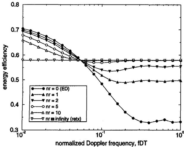
Fig. 3. Energy efficiency vs normalized Doppler bandwidth,  $f_D T$ . Parameterized retransmission ( $n_r = 0, 1, 2, 5, 10, \infty$ ).  $N = 10$ .  $g_d = 0.1$ ,  $b \rightarrow \infty$ .  $F = 5$  dB,  $\lambda = 1/N$ .
