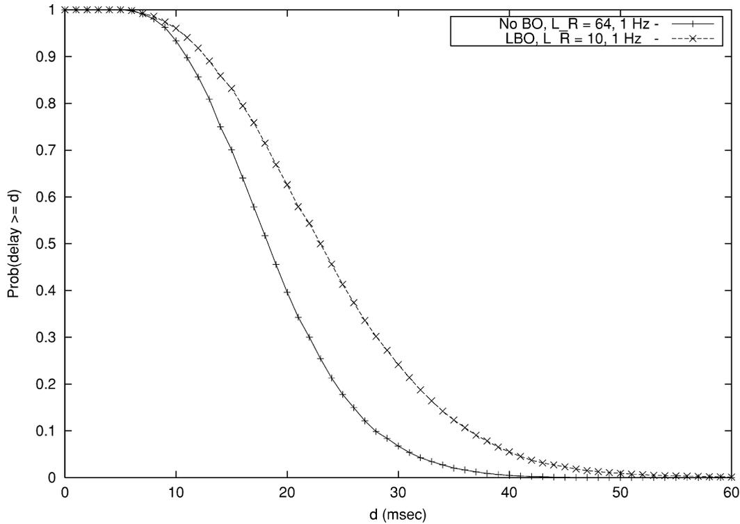
Fig. 12. Prob(delay  $\geq d$ ) versus  $d$  (ms) with and without BO.  $f_d = 1$  Hz. SNR = 5 dB.  $L_R = 64$  for no BO.  $L_R = 10$  for LBO.
