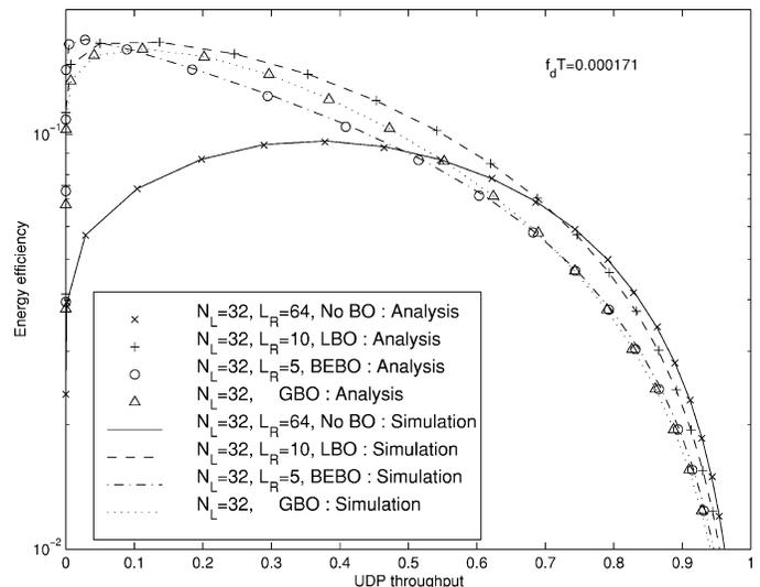
Fig. 6. Energy efficiency versus UDP throughput performance for no BO, LBO, BEBO and GBO.  $f_d T = 0.000171$ .  $g = 0.8$  for GBO.
