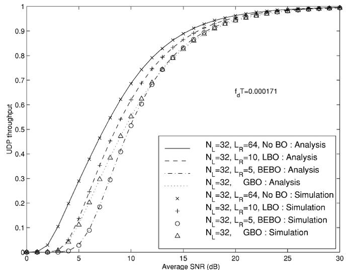
Fig. 5. Comparison of UDP throughput performance versus average SNR for no BO, LBO, BEBO, and GBO at the LL.  $f_d T = 0.000171$ .  $g = 0.8$  for GBO.
