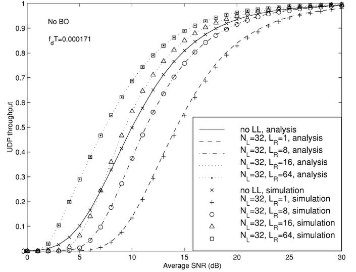
Fig. 3. UDP throughput performance with and without LL. LL has no backoff.  $N_U = 1024$  B.  $N_L = 32$ .  $L_R = 1, 8, 16, 64$ .  $f_d T = 0.000171$ .
