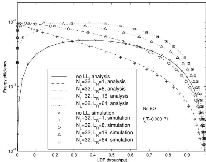
Fig. 4. Energy efficiency versus UDP throughput with and without LL. LL has no backoff.  $N_U = 1024$  B.  $N_L = 32$ .  $L_R = 1, 8, 16, 64$ .  $f_d T = 0.000171$ .
