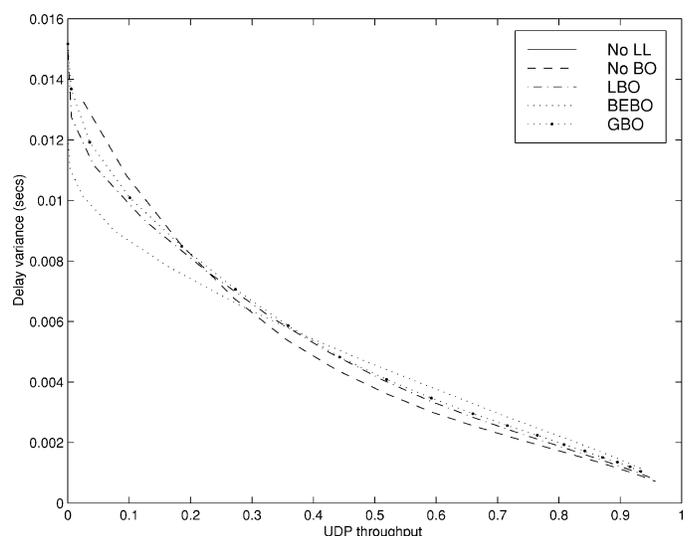
Fig. 11. Delay variance of voice packets versus UDP throughput performance for no LL, LL with no BO, LL with LBO, BEBO and GBO.  $f_d T = 0.000171$ .  $L_R = 64$  for No BO.  $L_R = 10$  for LBO,  $L_R = 5$  for BEBO.  $g = 0.8$  for GBO.
