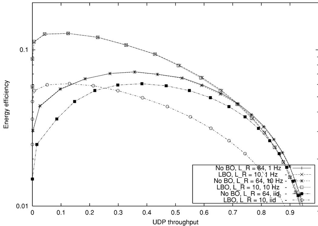
Fig. 8. Energy efficiency versus UDP throughput performance with and without backoff for varying fading correlations.  $f_d = 1$  Hz, 10 Hz, i.i.d.  $L_R = 10$  for LBO.  $L_R = 64$  for no BO.
