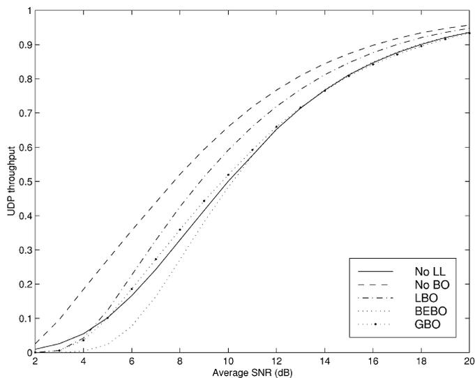
Fig. 9. UDP throughput versus average SNR performance for no LL, LL with no BO, LL with LBO, BEBO and GBO.  $f_d T = 0.000171$ .  $L_R = 64$  for No BO.  $L_R = 10$  for LBO,  $L_R = 5$  for BEBO.  $g = 0.8$  for GBO.
