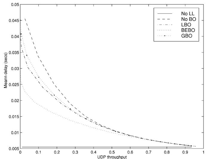
Fig. 10. Mean Delay of voice packets versus UDP throughput performance for no LL, LL with no BO, LL with LBO, BEBO and GBO.  $f_d T = 0.000171$ .  $L_R = 64$  for No BO.  $L_R = 10$  for LBO,  $L_R = 5$  for BEBO.  $g = 0.8$  for GBO.
