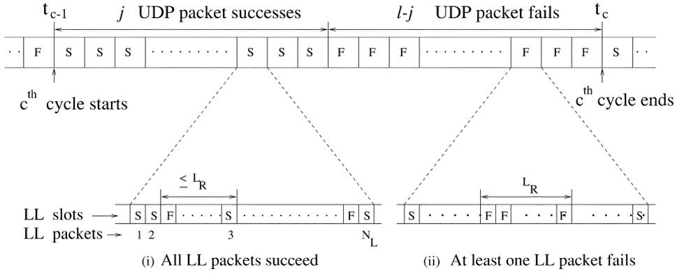
Fig. 2. UDP transmission cycle.
