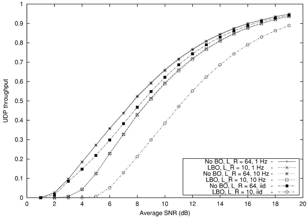
Fig. 7. UDP throughput versus average SNR performance with and without backoff for varying fading correlations.  $f_d = 1$  Hz, 10 Hz, i.i.d.  $L_R = 10$  for LBO.  $L_R = 64$  for no BO.
