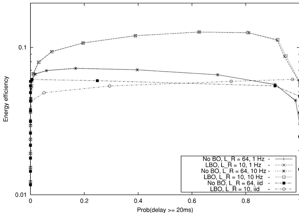
Fig. 13. Energy efficiency versus Prob(delay  $\geq$  20 s) with and without BO.  $f_d = 1$  Hz, 10 Hz, i.i.d.  $L_R = 10$  for LBO.  $L_R = 64$  for no BO.
