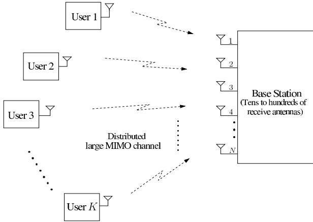
Fig. 1. An illustration of the uplink multiuser-user MIMO system with  $K$  transmitting users and  $N$  receiving antennas at the base station.
