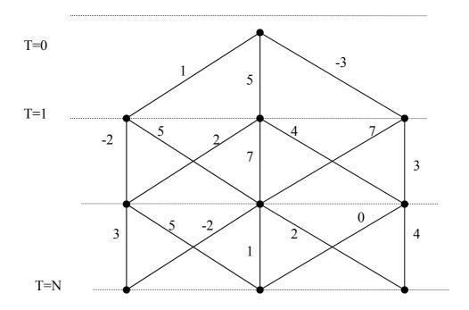
The number of different *paths* is exponential in N, so trying them all is not feasible. Instead, we can use backward recursion to compute the maximal distance from each node to the end step, staring with T=N.
