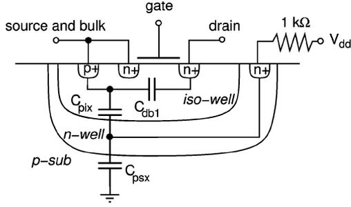
Fig. 7. Cross section of a triple-well device.
