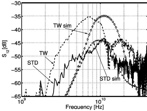
Fig. 16. Measured and simulated reverse isolation for STD and TW LNAs.
