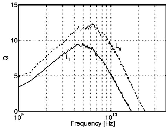
Fig. 17. Measured quality factor for gate and load inductors.
