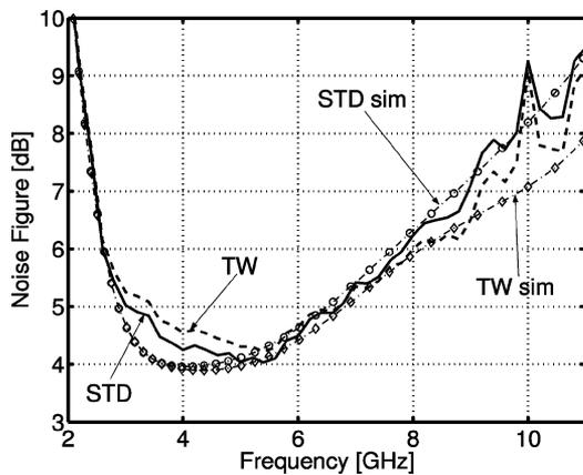
Fig. 18. Measured and simulated spot NF for STD and TW LNAs.
