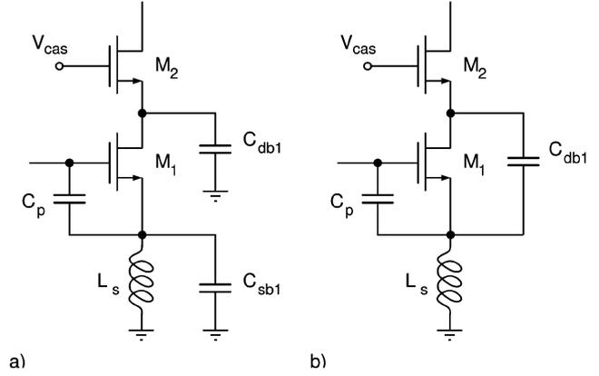
Fig. 5. Impact of parasitic capacitances. The bulk is (a) grounded and (b) connected to the source.
