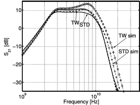
Fig. 14. Measured and simulated power gain for STD and TW LNAs.
