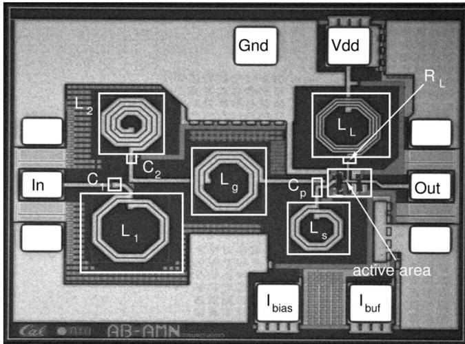
Fig. 11. Microphotograph of the LNA employing standard devices.
