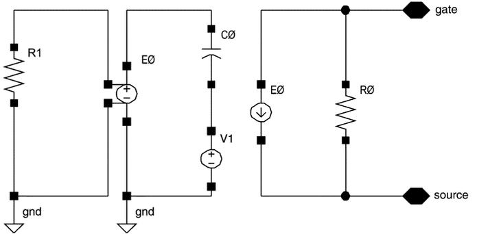
Fig. 19. Circuit model for inclusion of induced gate noise in the simulation.
