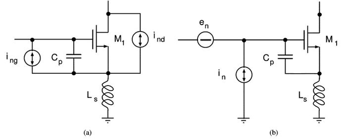
Fig. 8. Noise model for the amplifying transistor  $M_1$ . (a)  $M_1$  noise sources. (b) Input-referred equivalent noise generators.
