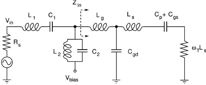
Fig. 4. Schematic of the LNA input network.
