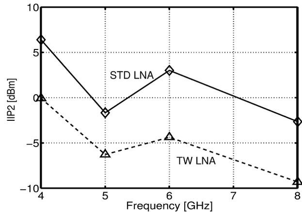
Fig. 21. Measured two-tone IIP2 for STD and TW LNAs.
