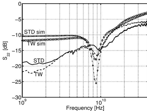
Fig. 13. Measured and simulated output reflection coefficient for STD and TW LNAs.
