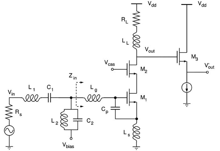
Fig. 3. Simplified schematic of a wideband LNA.
