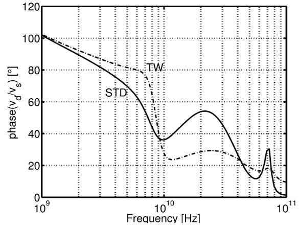
Fig. 6. Phase of the drain–source gain for the case of grounded bulk (solid line) and of bulk connected to the source of  $M_1$  (dash–dotted line).
