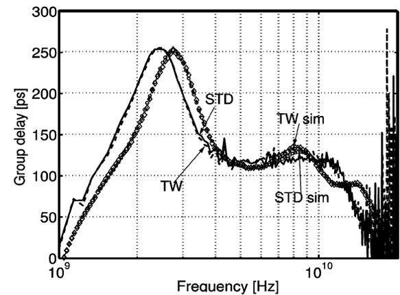
Fig. 15. Measured and simulated group delay for STD and TW LNAs.
