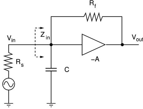
Fig. 2. Conceptual schematic of a shunt feedback amplifier.
