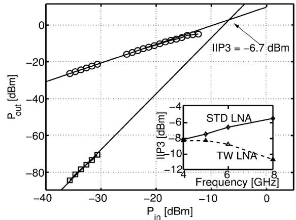
Fig. 20. Measured two-tone test at 6 GHz for STD and TW LNAs. Inset: Measured IIP3 versus frequency.
