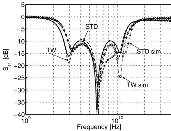
Fig. 12. Measured and simulated input reflection coefficient for STD and TW LNAs.
