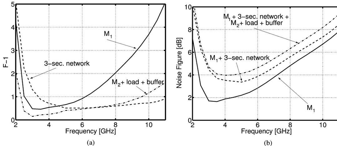
Fig. 10. Noise contributors of the designed LNA. (a) Noise contributions due to  $M_1$  (solid line), input network (dashed line), and  $M_2$ , load and  $M_3$  (dash-dotted line). (b) NF set by  $M_1$  only (solid line), by  $M_1$  and input network (dashed line), and by all circuit components (dash-dotted line).
