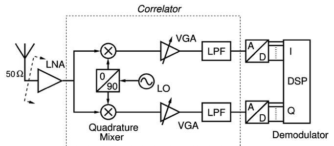
Fig. 1. Block diagram of a UWB receiver. The dashed box represents the subsystem that brings the RF signal to baseband in order to recover the information signal: it can be a correlation filter followed by a sampler or, as depicted here as an example, a quadrature mixer.
