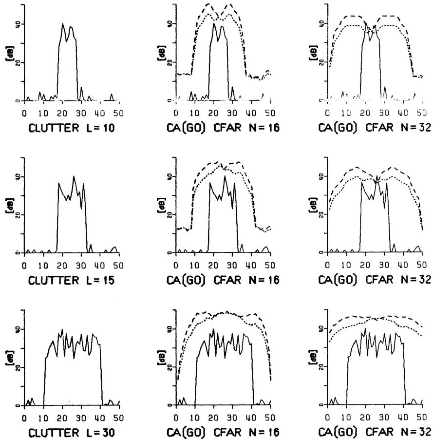
Fig. 6. Some examples for the CA and CAGO CFAR behavior in model 2 clutter situations with uniformly distributed statistically independent clutter amplitudes and different clutter area lengths  $L$ . Dotted lines show the threshold response for CA CFAR and dashed lines for CAGO CFAR.
