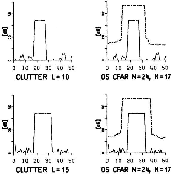
Fig. 11. Behavior of OS CFAR ( $N = 24$ ,  $k = 17$ ) in model 2 clutter situations with fully correlated clutter amplitudes (deterministic model).
