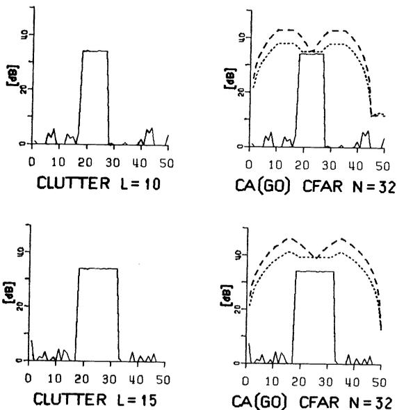
Fig. 7. Behavior of CA and CAGO CFAR in model 2 clutter situations with fully correlated clutter amplitudes and different clutter area lengths  $L$ , dotted and dashed lines as in Fig. 6.
