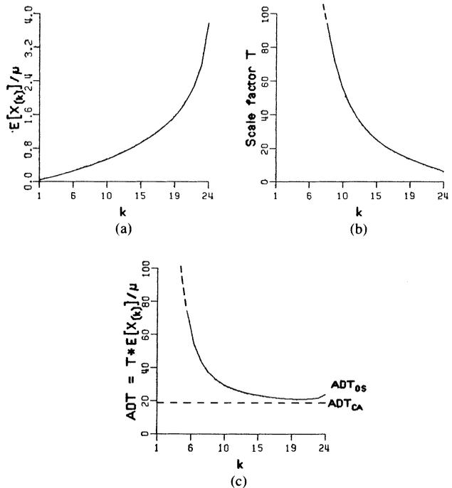
Fig. 8. (a) Mean value  $E(X_{(k)})/\mu$  of the random variable  $X_{(k)}$  for  $N = 24$ . (b) Scaling factor  $T$  for the OS CFAR and  $P_{fa} = 10^{-6}$ ,  $N = 24$ . (c) Average decision threshold ADT given in (1) for OS CFAR with  $N = 24$  and  $P_{fa} = 10^{-6}$ . For reference the ADT for CA CFAR with the same reference window size  $N = 24$  is shown by the dashed line.
