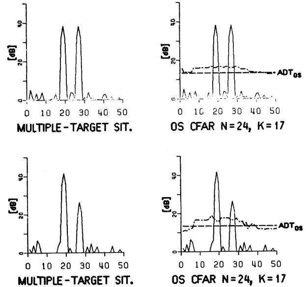
Fig. 12. Behavior of OS CFAR ( $N = 17$ ) in the same model 3 double target situation as in Fig. 3.
