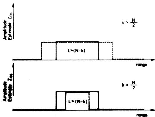
Fig. 10. Principal impact of the rank-order parameter  $k$  on the clutter power estimation in OS CFAR. The clutter power is shown in solid lines and the clutter power estimation  $Z$  in dotted lines. For  $k > N/2$  the clutter area appears extended (dilatation), for  $k < N/2$  it appears shrunk (erosion).
