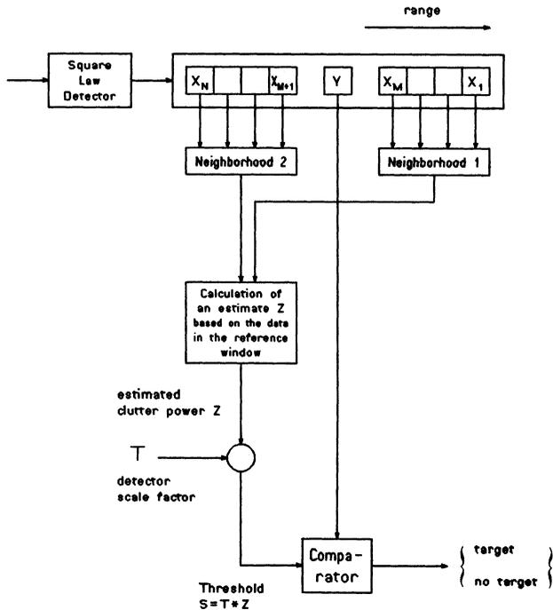
Fig. 1. General CFAR processor. The central operation of the CFAR system is to estimate the clutter power level  $Z$ .
