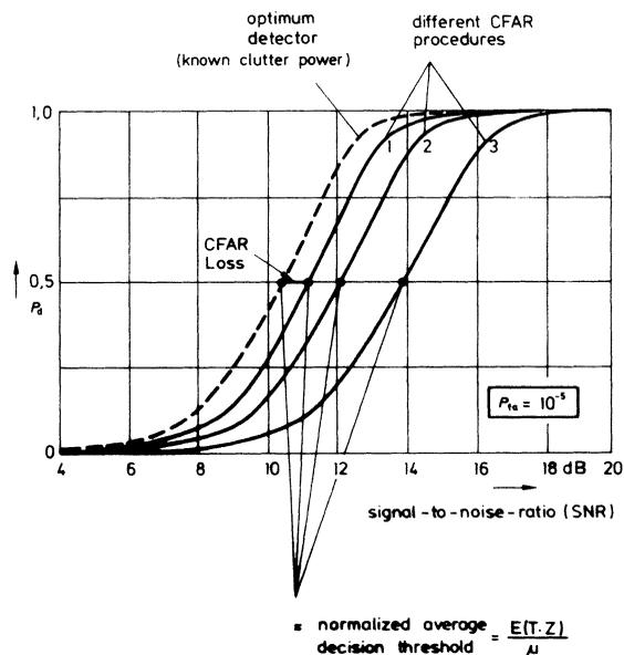
Fig. 5. Explanation of the performance measure ‘‘average decision threshold’’ ADT by means of the usual  $P_d$  SNR diagrams. The SNR of the minimum detectable signal ( $P_d = 0.5$ ) is approximately the same as the  $\text{ADT} = E(TZ)/\mu$  of each CFAR system. The random variable  $Z$  is the result of the clutter level estimation (see Fig. 1),  $T$  is the scaling factor controlling  $P_{fa}$ ,  $\mu$  is the actual mean clutter power level, and  $E$  stands for the expectation.
