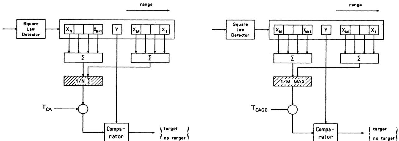
Fig. 2. Comparison of CA and CAGO CFAR procedures.
