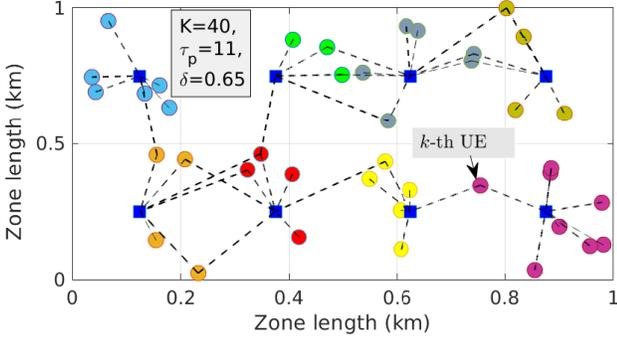
Fig. 1. A realization of the system model. The blue squares denote the AP positions and solid circles denote the UEs.
