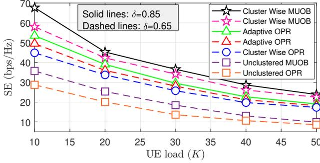
Fig. 4. Pilot length optimized SE vs. UE load ( $K$ ).
