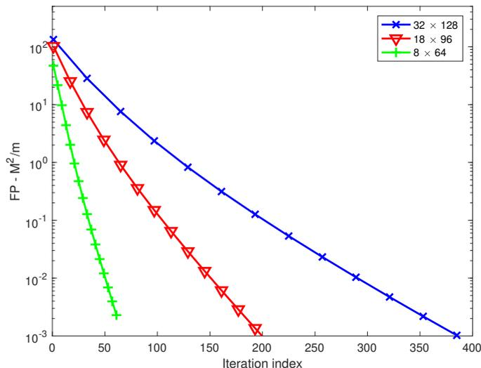
Figure 1: Difference between the FP of the algorithm and the optimal FP, as a function of the iteration index, for normalized UMTFs of size  $8 \times 64$ ,  $18 \times 96$  and  $32 \times 128$ .
