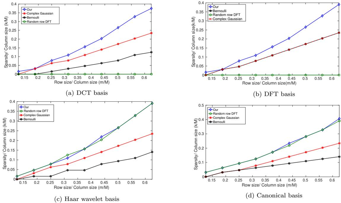
Figure 3: Comparison of the matrices constructed using our method, complex Gaussian random, Bernoulli random and partial DFT matrices through the phase transition characteristics.
