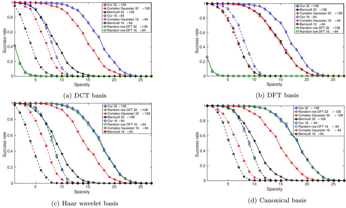
Figure 2: Comparison of the reconstruction performances of the matrices constructed from our method, complex Gaussian random, Bernoulli random and partial DFT matrices of size  $16 \times 64$  and  $32 \times 128$  by the OMP algorithm in different sparsifying bases.
