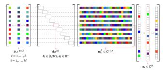
Measurement model at sensor I
