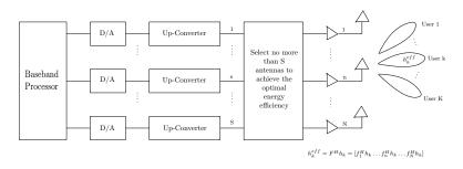
Figure: Virtual Multiuser Communication System
