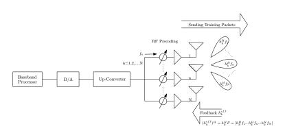
Figure: Beam-sweep Procedure
