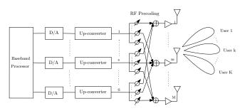
The system is consists of a baseband processor, digital-to-analog converter (DAC), upconverter, S RF chains, M transmit antennas, and K number of users.
