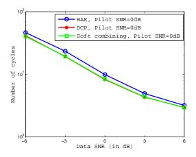
• At low to intermediate pilot SNRs, DCP-based scheme has better average hitting time performance
