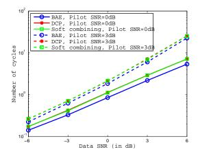
At low to intermediate pilot SNRs, DCP-based scheme performs better
