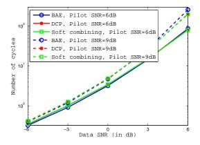
At high pilot SNRs, broadcast-based LMMSE scheme has better performance
