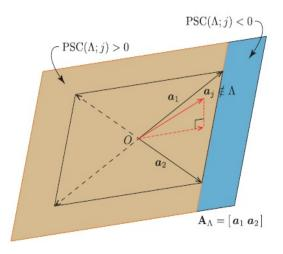
• *H*: hyperplane through  $a_j$ ,  $j \in \Lambda$ PSC $(\Lambda, j) > 0$  when orthogonal projection of  $a_j$  onto column space of  $A_{\Lambda}$  is on the same side of *H* as the origin
