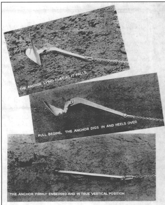
Fig 2. Photographs of the anchor showing the way in which it digs itself into the sea-bed like a plough-share regardless of the way it falls.
