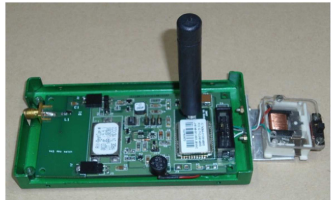
Fig. 9. The fabricated harvester board. The RF power is received by an external antenna connected through SMA port. The antenna shown is for the wireless radio.
