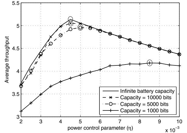
Fig. 4. Zoomed-in view of the average throughput as a function of  $\eta$  ( $E_s = 25000$ ,  $\rho = 0.01$ , and  $\bar{P}_{\text{EH}} = 250$ ). The peak value of every curve is encircled.
