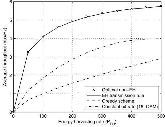
Fig. 1. Average throughput as a function of the average energy harvesting rate ( $\rho = 0.01$  and  $E = P_{\text{EH}}/\rho$ ).
