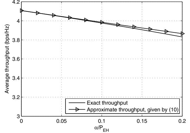
Fig. 3. Zoomed-in view of average throughput as a function of the energy overhead relative to average energy harvesting rate ( $\bar{P}_{\text{EH}} = 100$ ).
