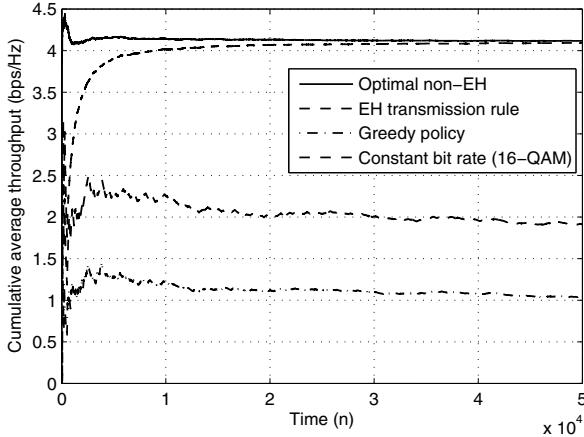
Fig. 2. Cumulative average of throughput as a function of time ( $E_s = 10000$ ,  $\rho = 0.01$ , and  $\bar{P}_{\text{EH}} = 100$ ).
