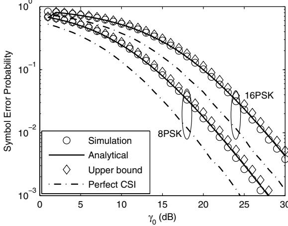
Fig. 1. SEP of cascaded channel estimation for 8PSK and 16PSK constellations ( $\bar{\gamma}_{sr} = \bar{\gamma}_{rd} = \bar{\gamma}_{sd} = \gamma_0$  and  $\varepsilon = 1$ )
