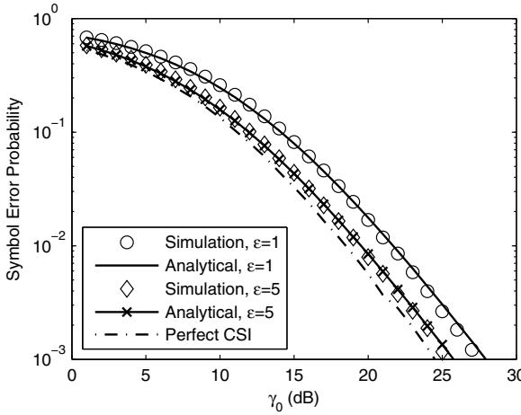
Fig. 2. SEP of cascaded channel estimation for different pilot power boosting factors,  $\varepsilon$  (8PSK and  $\bar{\gamma}_{sr} = \bar{\gamma}_{rd} = \bar{\gamma}_{sd} = \gamma_0$ )
