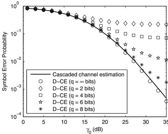
Fig. 3. Comparison of SEP of cascaded channel estimation and disintegrated channel estimation (D-CE) (16PSK,  $\bar{\gamma}_{sr} = \bar{\gamma}_{rd} = \bar{\gamma}_{sd} = \gamma_0$ , and  $\varepsilon = 1$ )
