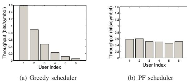
Fig. 4. Comparison of the throughputs of different UEs for the PF and greedy schedulers.
