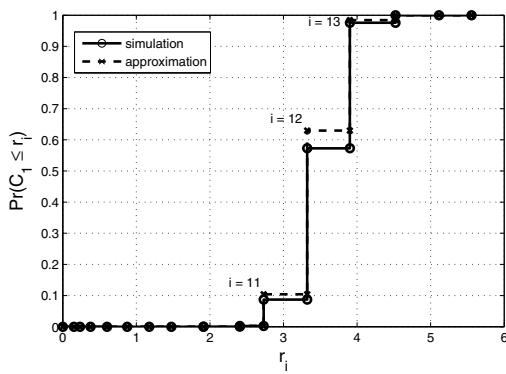
Fig. 1. Plot of the approximate cdf of  $C_1$  and the cdf generated from simulations ( $S = 4$ ,  $M = 2$ ,  $\sigma_1^2 = 13$  dB).
