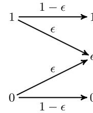
Fig. 1. A bit-wise *iid* binary symmetric erasure channel with erasure probability  $\epsilon$ , where the erased bit is denoted by  $e$ .
