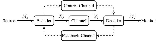
Fig. 2. An abstract discrete time communication model for a source, where the state  $M_j$  at time  $t = (j - 1)n + 1$  is encoded to an  $n$ -length codeword  $X_j$ , which is received as channel output  $Y_j$  after  $n$  channel uses at time  $t = jn + 1$ . Decoder forms an estimate  $\hat{M}_j$  at the reception instant, where each transmitted bit is erased independently and identically.
