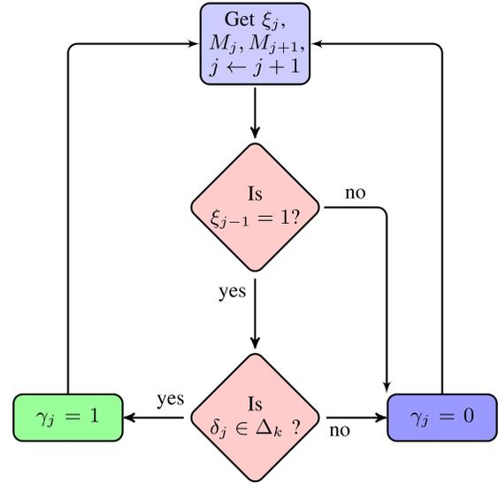
Fig. 3. We show the flow chart for the algorithm used by the source in generalized incremental update scheme, to encode message  $M_j$  as incremental or true update.
