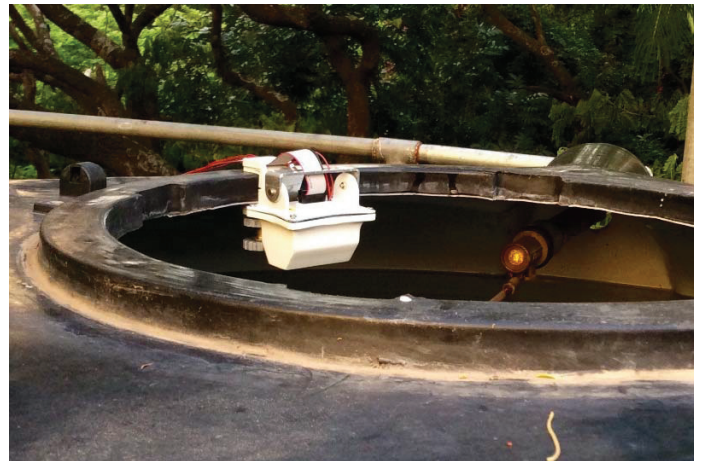
Fig. 9. Installation on a tank. The sensor transducer block is attached to the rim and freely hangs to ensure a vertical direction.
