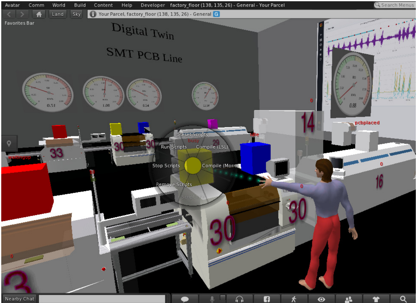
Fig. 4: Visualization of concurrent DTs. Also shown is a virtual human avatar interacting with the line using HMI panels
