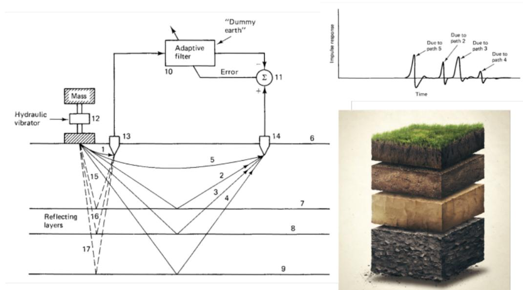
Seismic impulse response for subsurface imaging ("layer identification").
