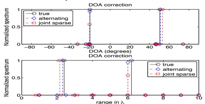
Fig. 4: Grid matching: sources located at  $(50.4^\circ, 2.4\lambda)$  and  $(-20.6^\circ, 6.2\lambda)$ . The estimated DOA from step-1 is refined, and it is then used for range estimation.
