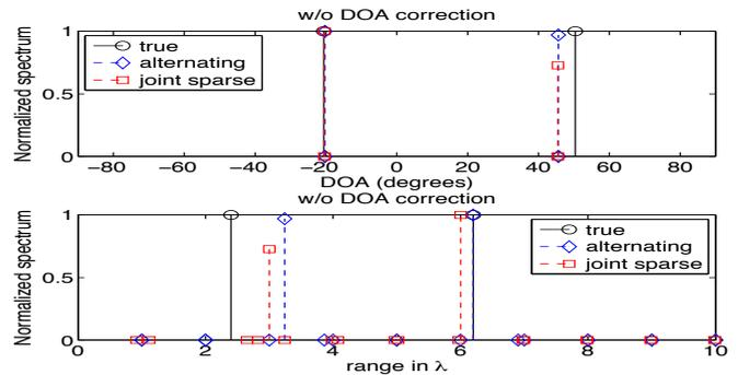
Fig. 3: Grid matching: sources located at  $(50.4^\circ, 2.4\lambda)$  and  $(-20.6^\circ, 6.2\lambda)$ . The estimated DOA from step-1 is used for range estimation without any correction.
