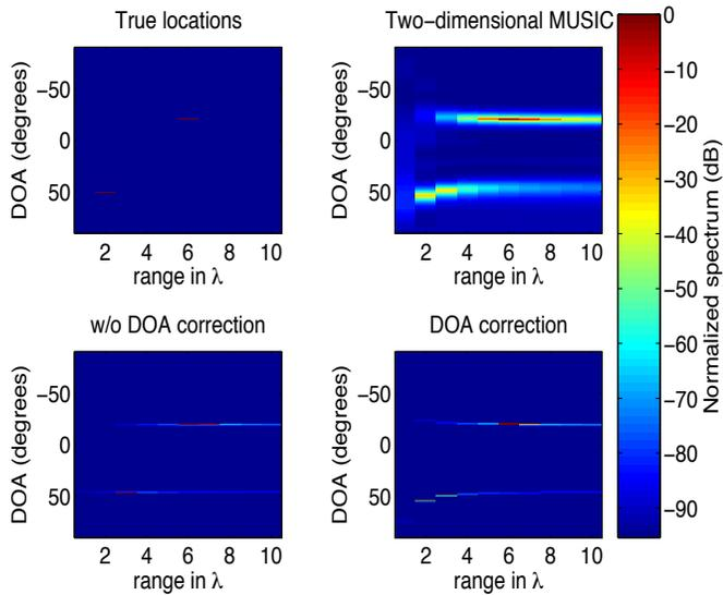
Fig. 2: Ignoring the grid mismatch: Sources located in the near-field at  $(50.4^\circ, 2.4\lambda)$  and Fresnel region at  $(-20.6^\circ, 6.2\lambda)$ .
