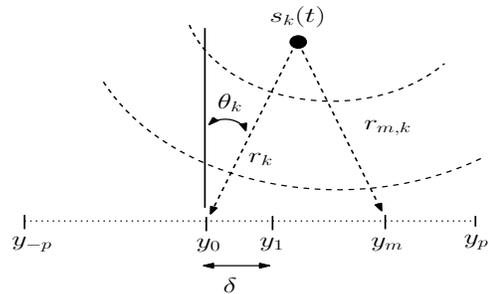
Fig. 1: A linear array receiving a signal from a near-field source.
