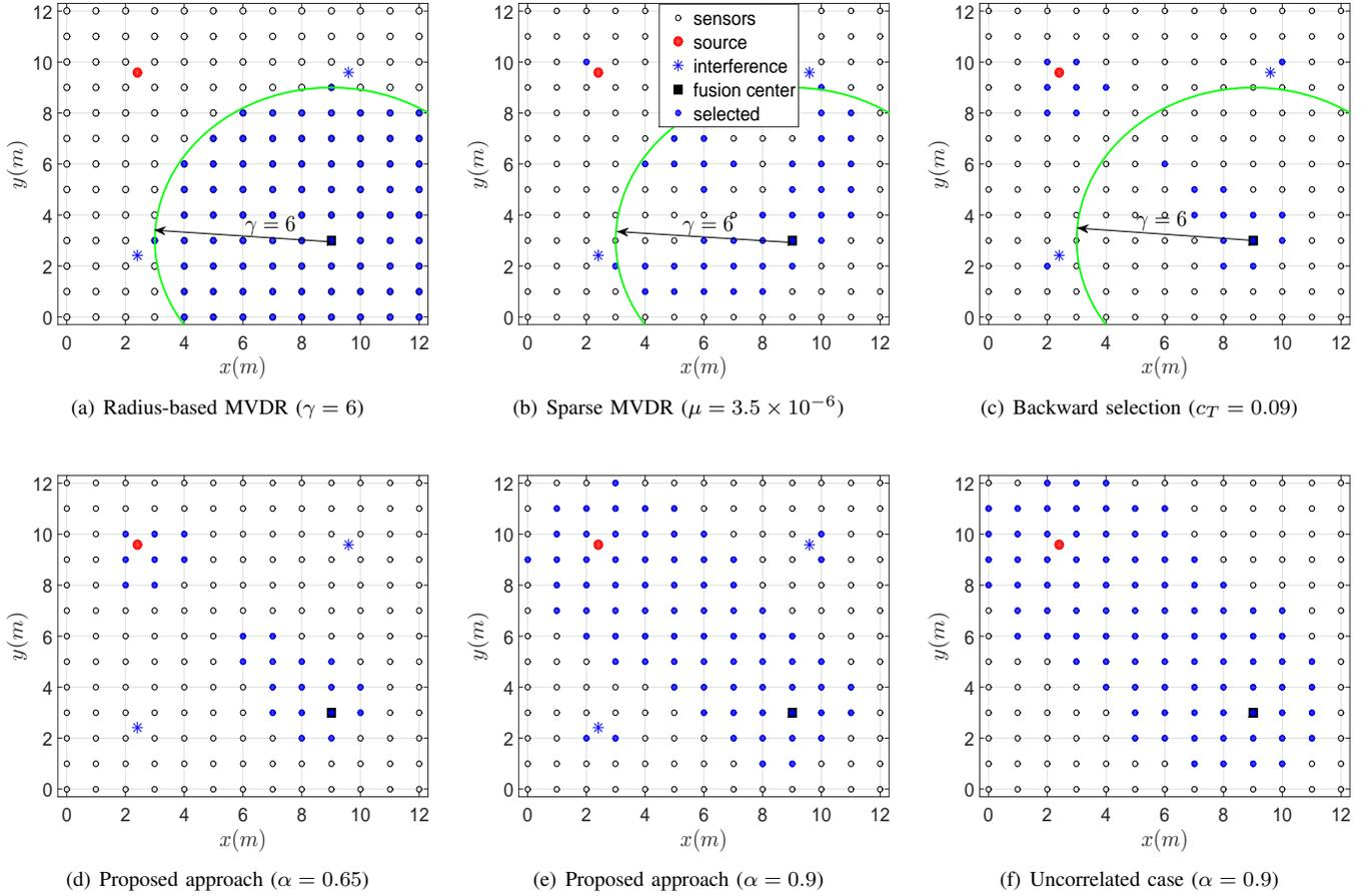
Figure 2. Microphone subset selection examples (The blue sensors are activated for the MVDR beamformer): (a) radius-based MVDR beamforming, (b) sparse MVDR beamforming, (c) backward selection [20] and (d) proposed method ( $\alpha = 0.65$ ) for spatially correlated noises, respectively, (e) proposed method for correlated case with  $\alpha = 0.9$ , and (f) proposed method ( $\alpha = 0.9$ ) for spatially uncorrelated noises only.
