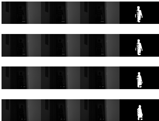
Figure: Original, V-BM-3D, K-SVD, ReProCS. In the video, a person is walking through a hallway. ReProCS successfully “sees” the person.
