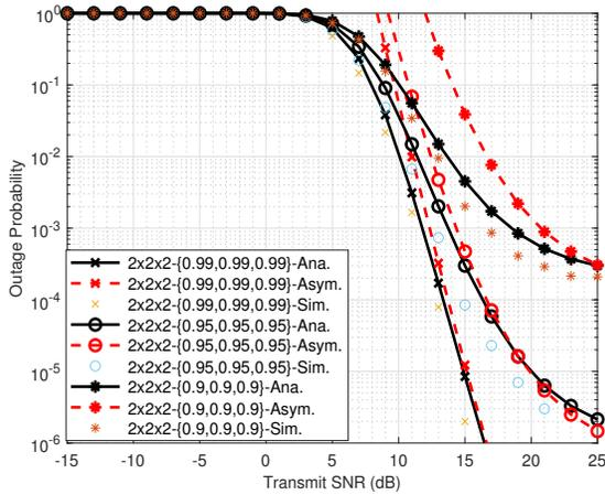
**Fig. 2** Outage probability analysis of  $2 \times 2 \times 2$  MIMO antenna configurations under different CEE conditions with  $\alpha = 0.2$ .
