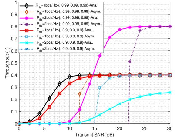
**Fig. 4** Throughput analysis of  $2 \times 2 \times 1$  MIMO antenna configurations for different threshold rates under different imperfect CSI conditions.
