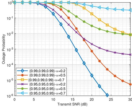
**Fig. 3** Outage probability analysis of  $2 \times 1 \times 2$  MIMO antenna configurations for perfect and imperfect CSI for different  $\alpha$  values.
